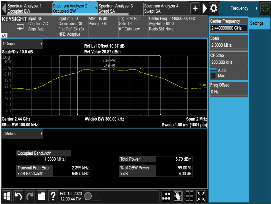
Figure 8 - 2440 MHz – Emission Bandwidth
