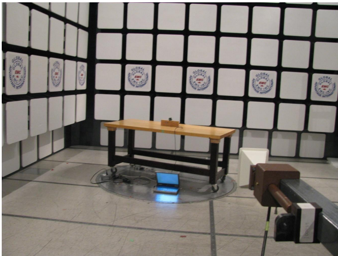
Figure 2 – Radiated emission setup
