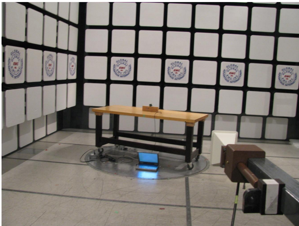
Figure 2 – Radiated emission setup
