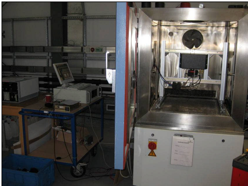
Picture 10: Test set-up dry heat (dry heat storage)
