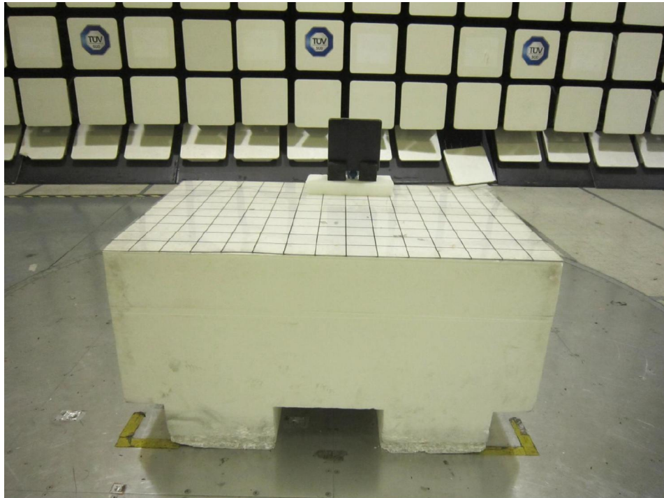
Radiated Emissions Test Setup (Front View)
