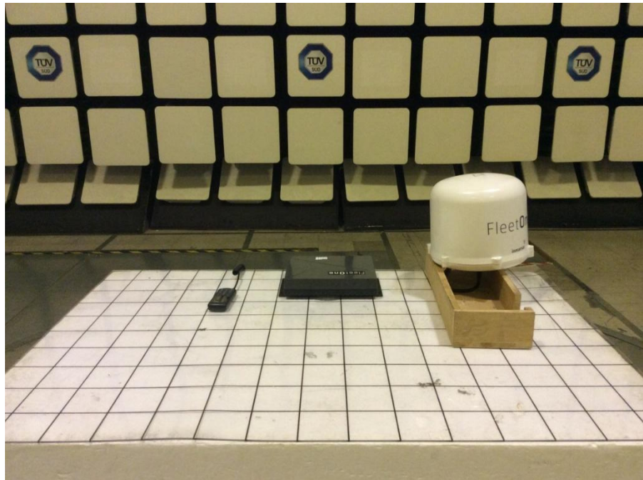
Radiated Spurious Emissions Test Setup (Front View)
