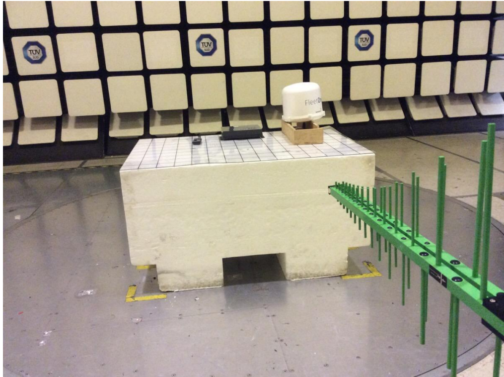
Radiated Emissions Test Setup (Front View)
