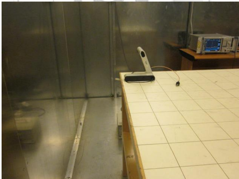
Conducted Emissions Test Setup (Rear View)
