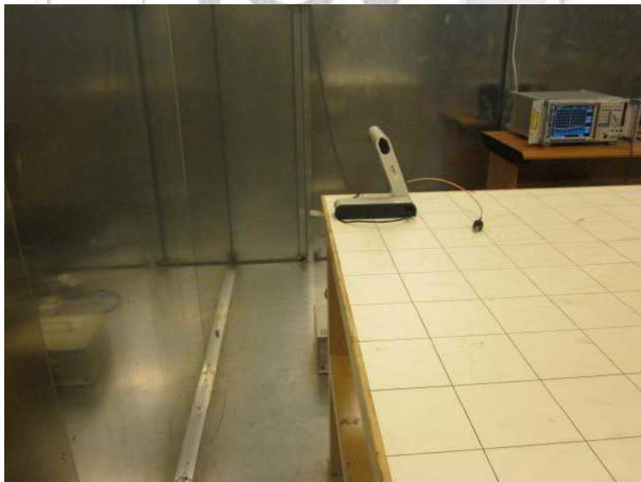
Conducted Emissions Test Setup (Rear View)
