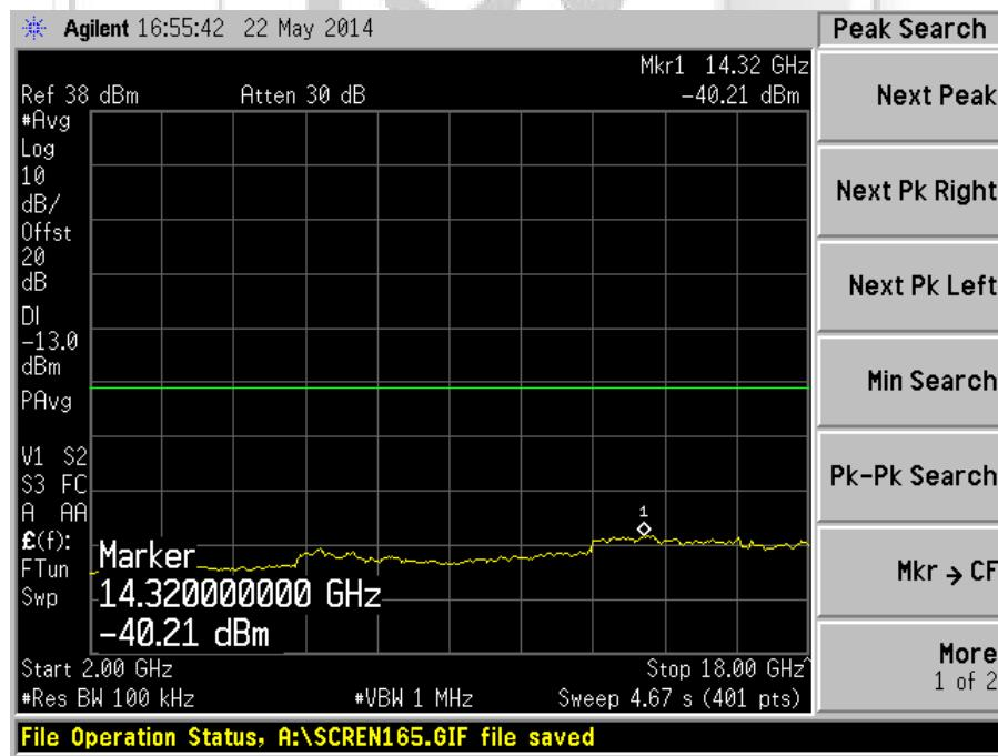
UNWANTED EMISSIONS AT ANTENNA TERMINAL TEST
