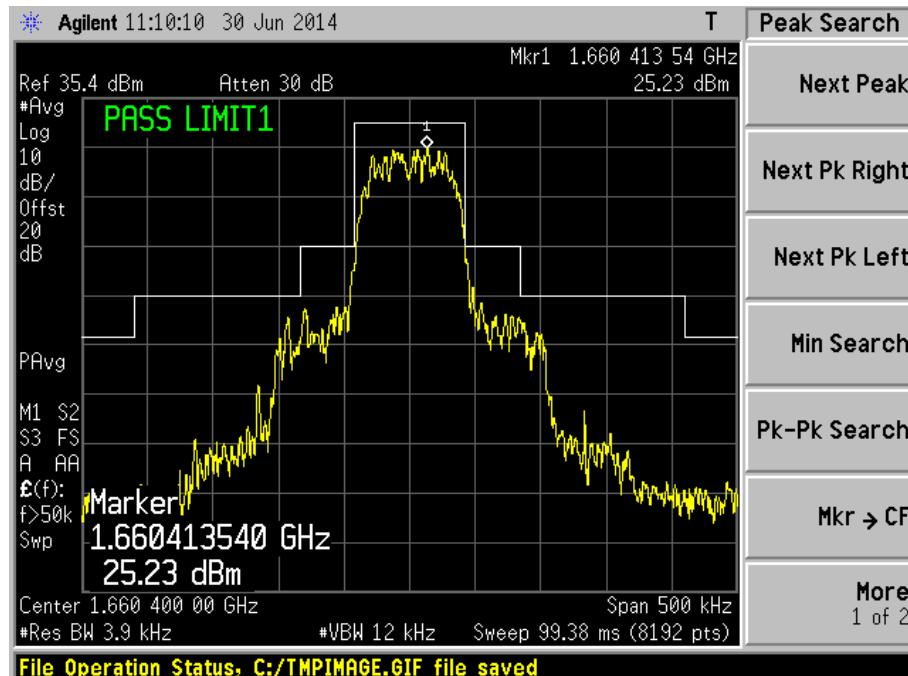
UNWANTED EMISSIONS AT ANTENNA TERMINAL TEST
