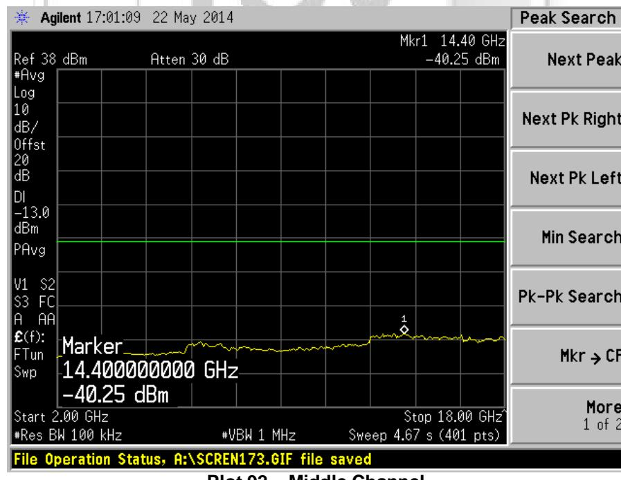
**UNWANTED EMISSIONS AT ANTENNA TERMINAL TEST**
