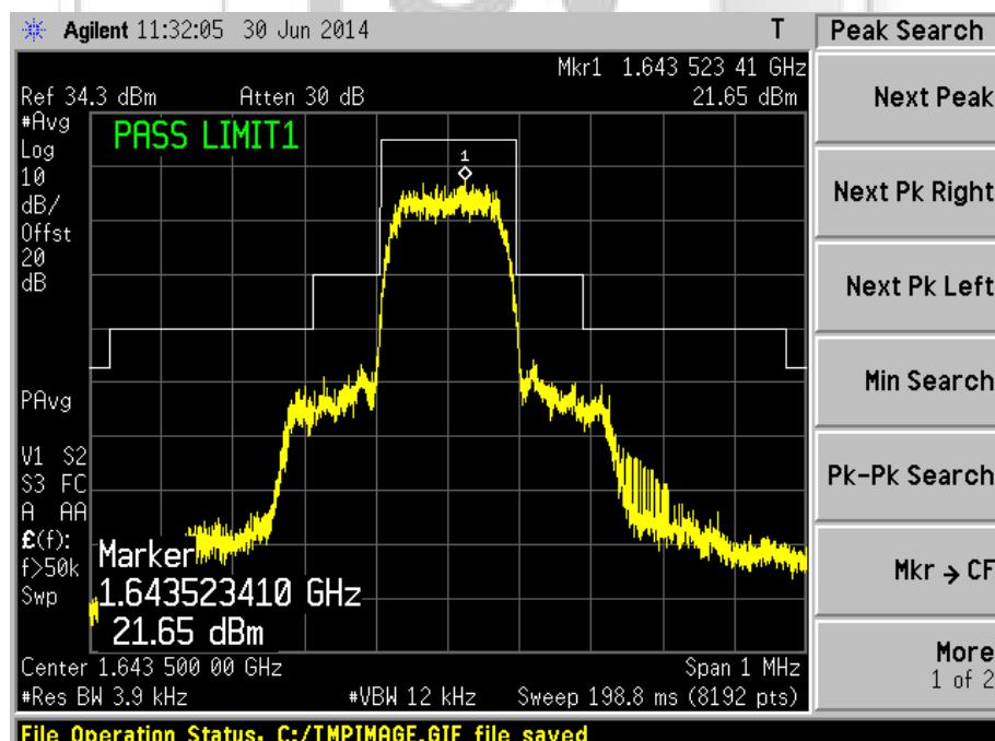
**UNWANTED EMISSIONS AT ANTENNA TERMINAL TEST**
