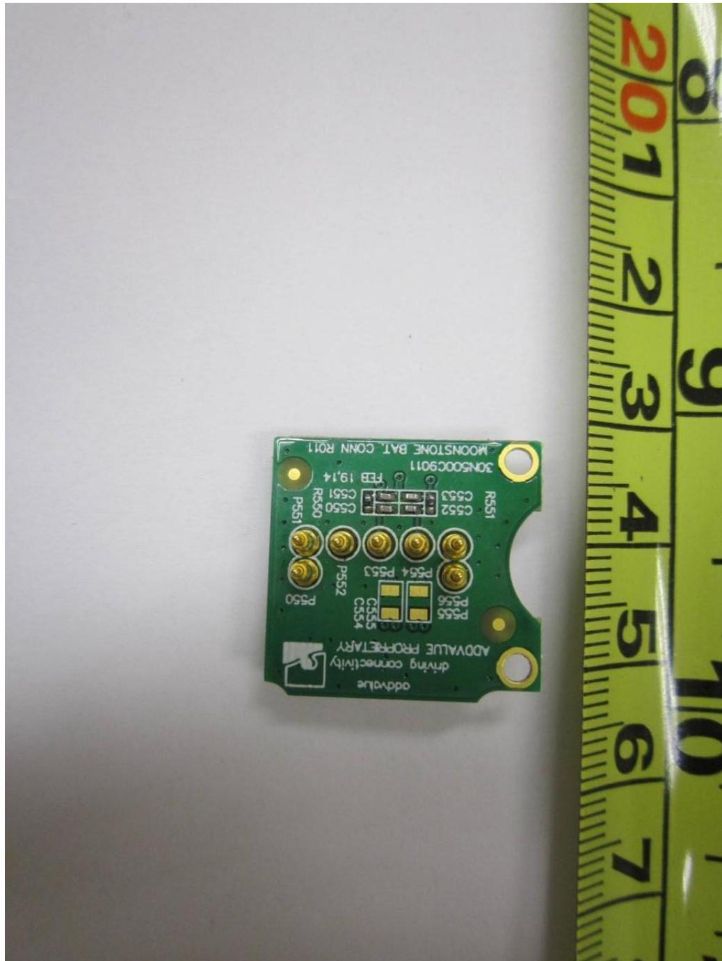
**Battery Contact PCBA Trace Side**
