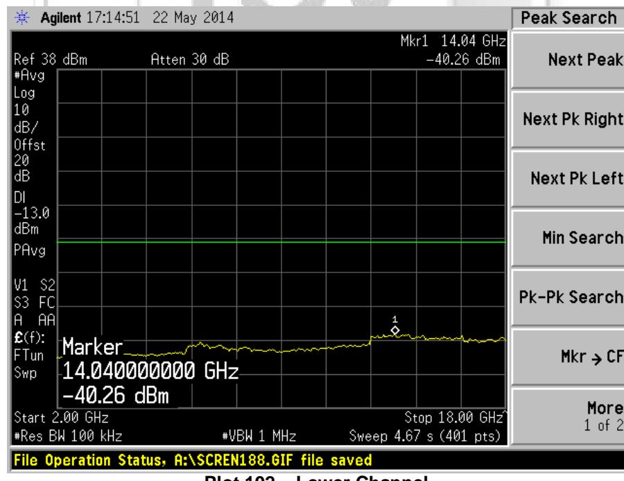
UNWANTED EMISSIONS AT ANTENNA TERMINAL TEST
