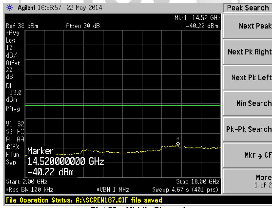
**UNWANTED EMISSIONS AT ANTENNA TERMINAL TEST**
