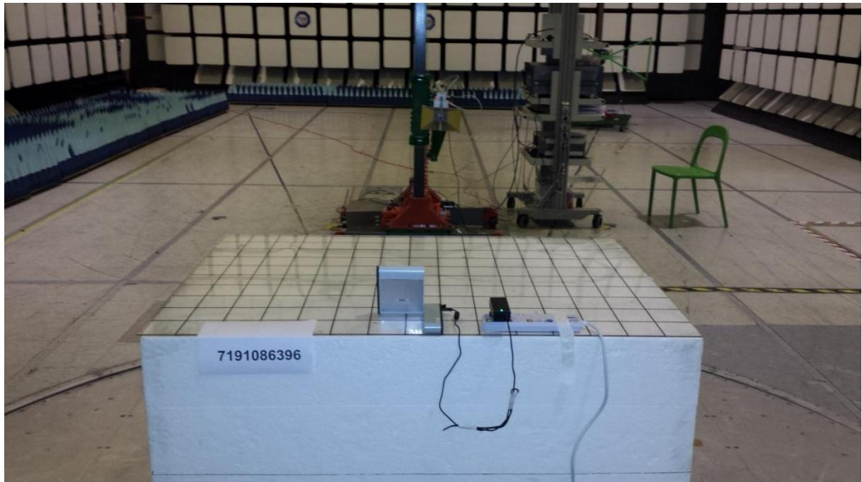
Radiated Spurious Emissions Test Setup (Front View)
