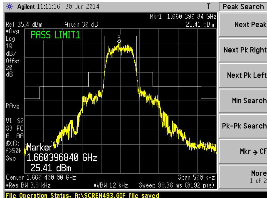
UNWANTED EMISSIONS AT ANTENNA TERMINAL TEST
