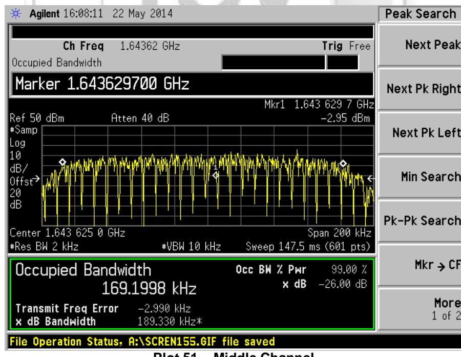
UNWANTED EMISSIONS AT ANTENNA TERMINAL TEST
