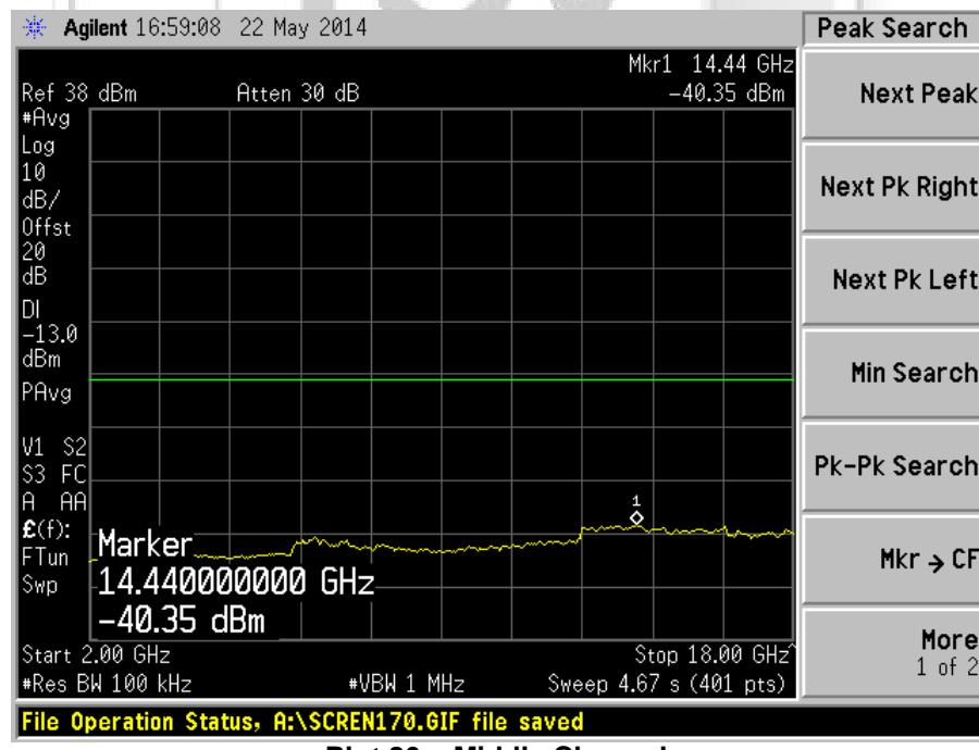
UNWANTED EMISSIONS AT ANTENNA TERMINAL TEST
