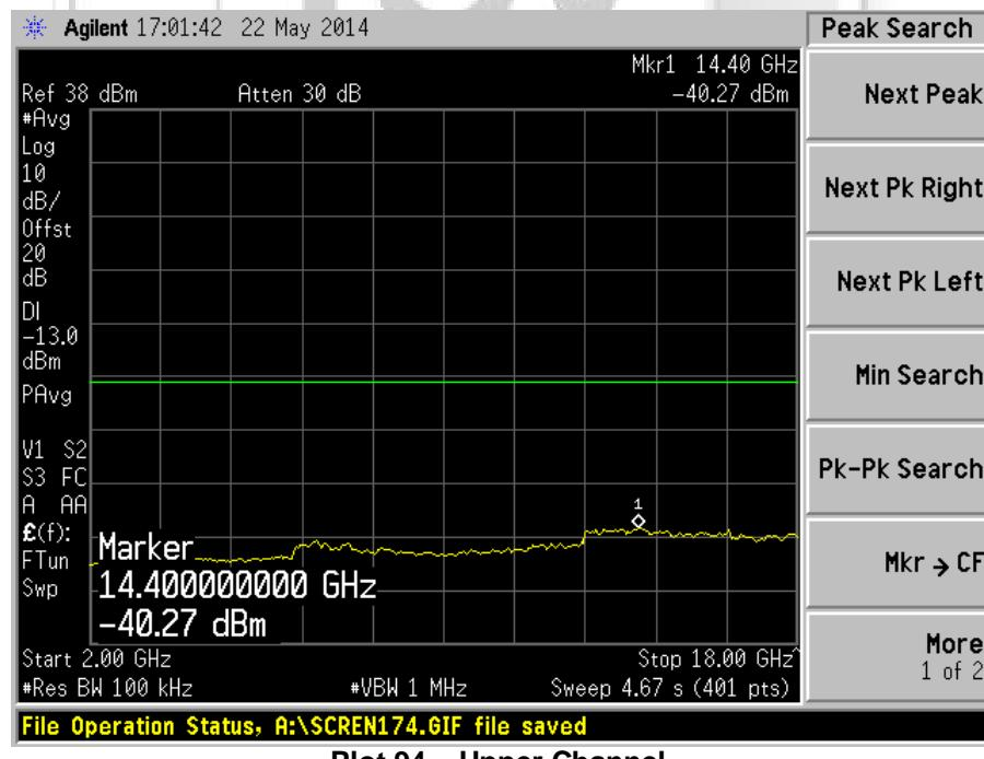
UNWANTED EMISSIONS AT ANTENNA TERMINAL TEST
