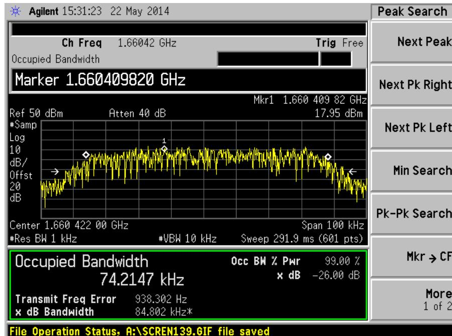
UNWANTED EMISSIONS AT ANTENNA TERMINAL TEST
