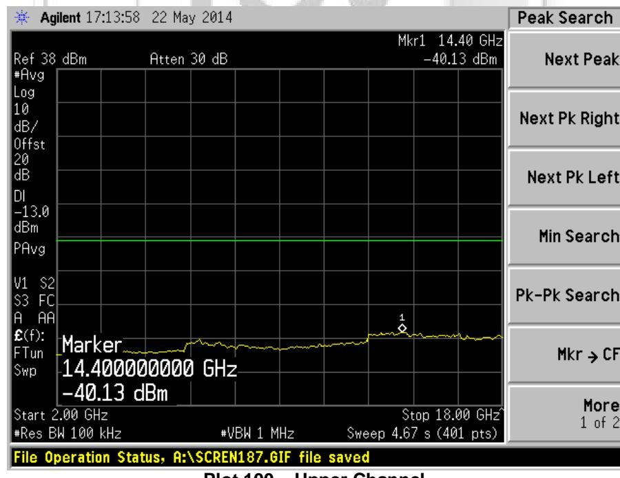
UNWANTED EMISSIONS AT ANTENNA TERMINAL TEST
