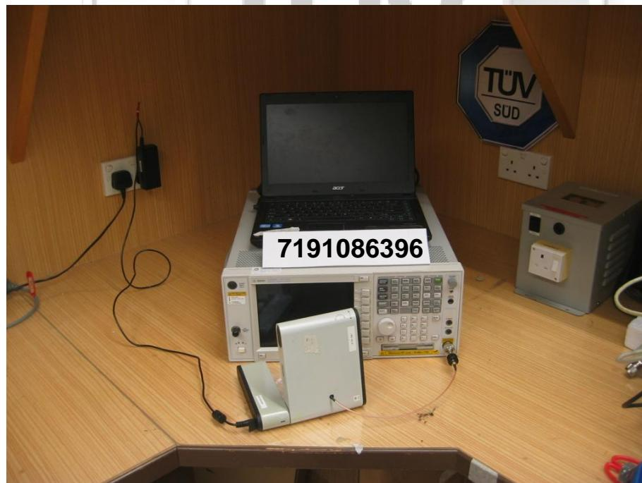
Unwanted Emissions at Antenna Terminal Test Setup
