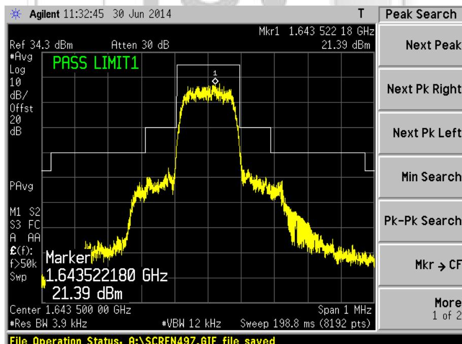
UNWANTED EMISSIONS AT ANTENNA TERMINAL TEST
