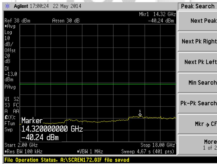
UNWANTED EMISSIONS AT ANTENNA TERMINAL TEST
