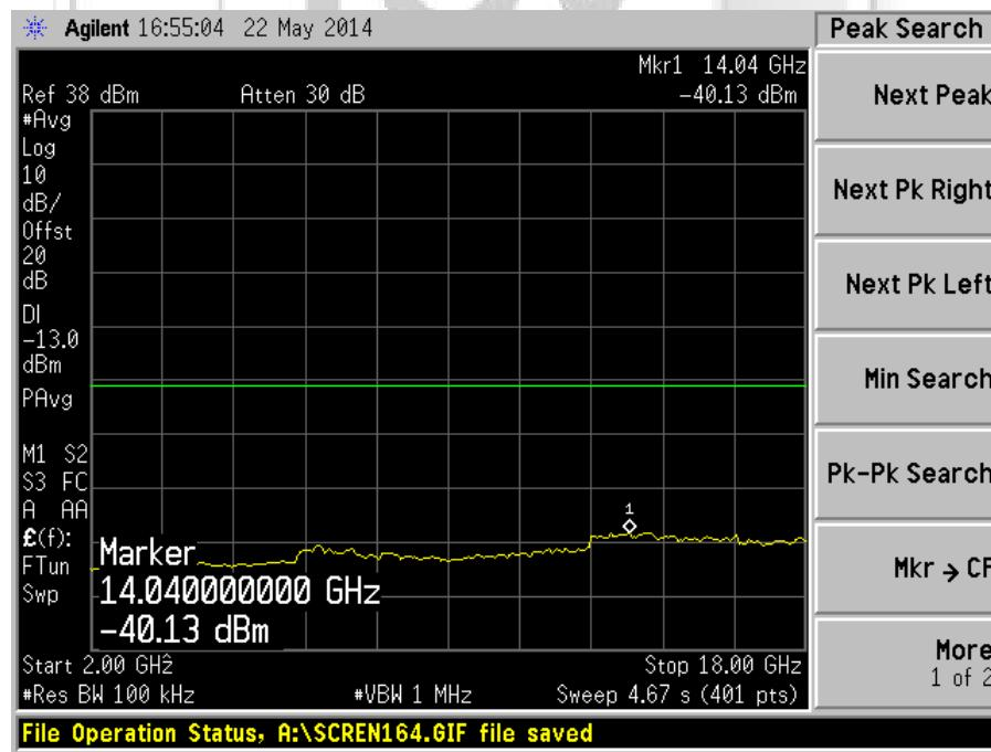
UNWANTED EMISSIONS AT ANTENNA TERMINAL TEST
