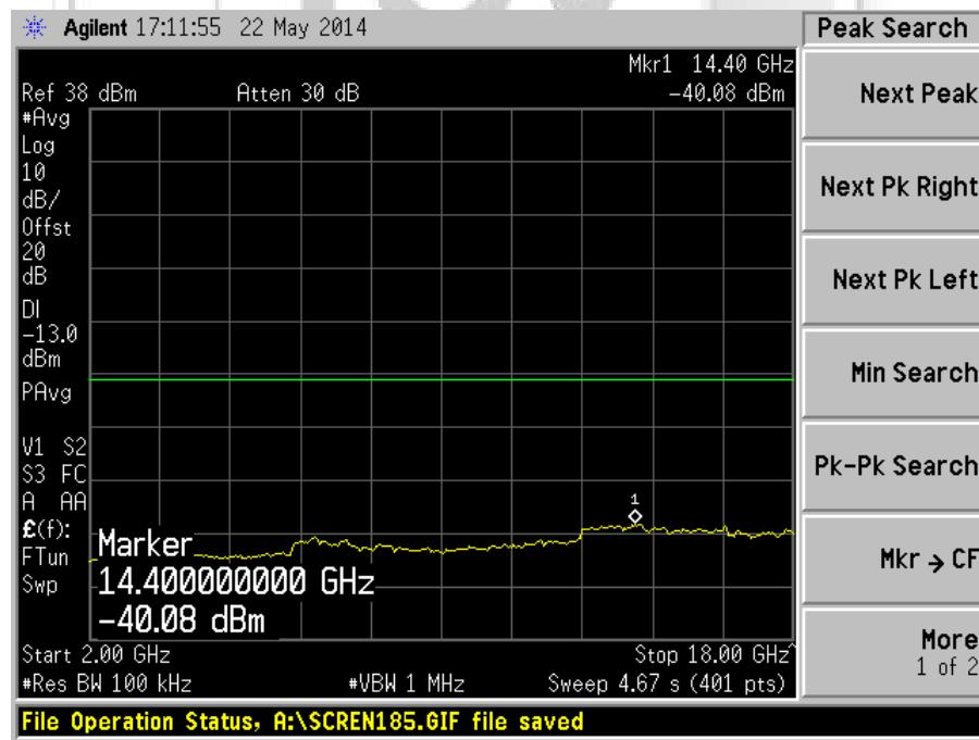
UNWANTED EMISSIONS AT ANTENNA TERMINAL TEST
