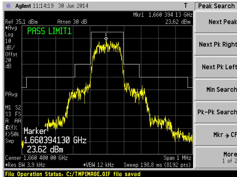
UNWANTED EMISSIONS AT ANTENNA TERMINAL TEST
