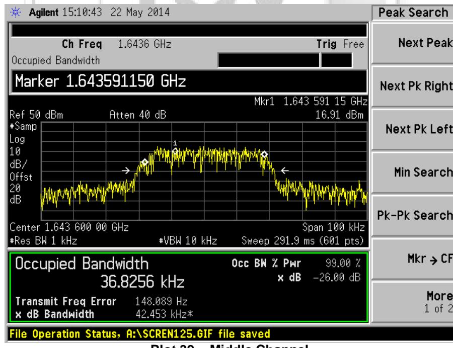
**UNWANTED EMISSIONS AT ANTENNA TERMINAL TEST**
