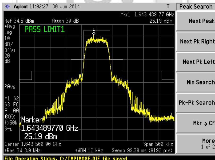
**UNWANTED EMISSIONS AT ANTENNA TERMINAL TEST**
