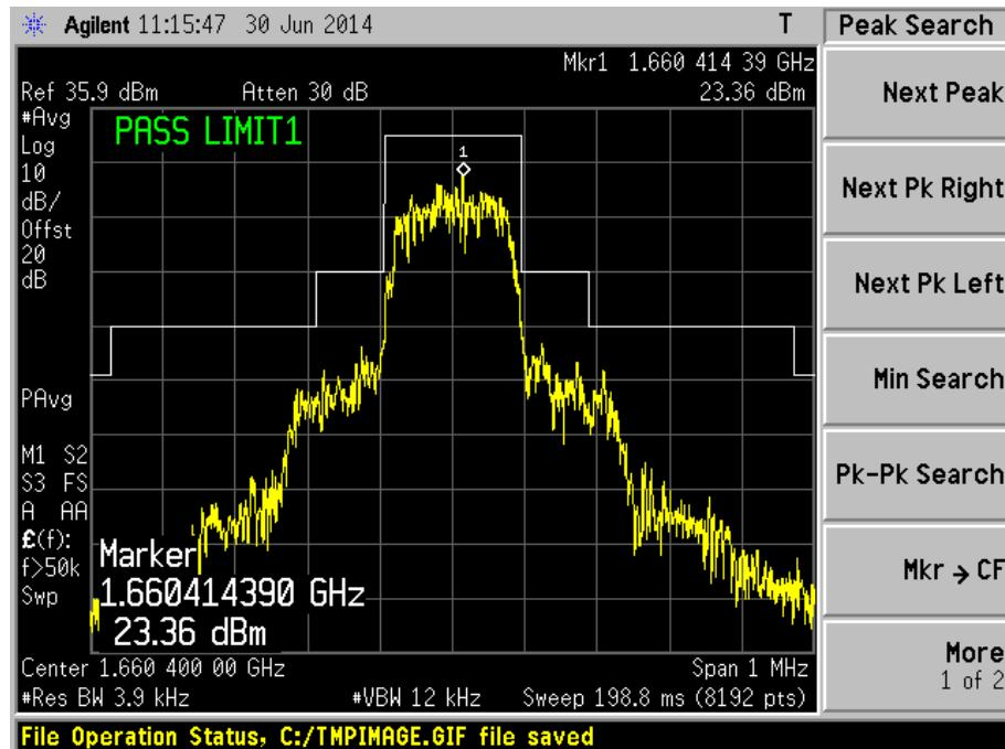
UNWANTED EMISSIONS AT ANTENNA TERMINAL TEST
