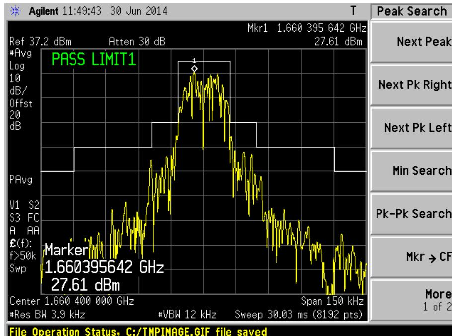
UNWANTED EMISSIONS AT ANTENNA TERMINAL TEST
