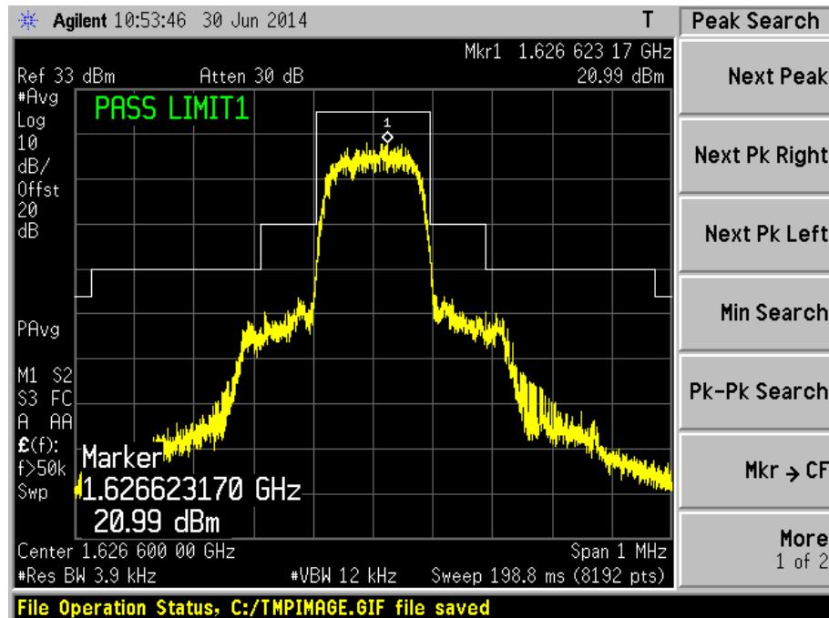
UNWANTED EMISSIONS AT ANTENNA TERMINAL TEST
