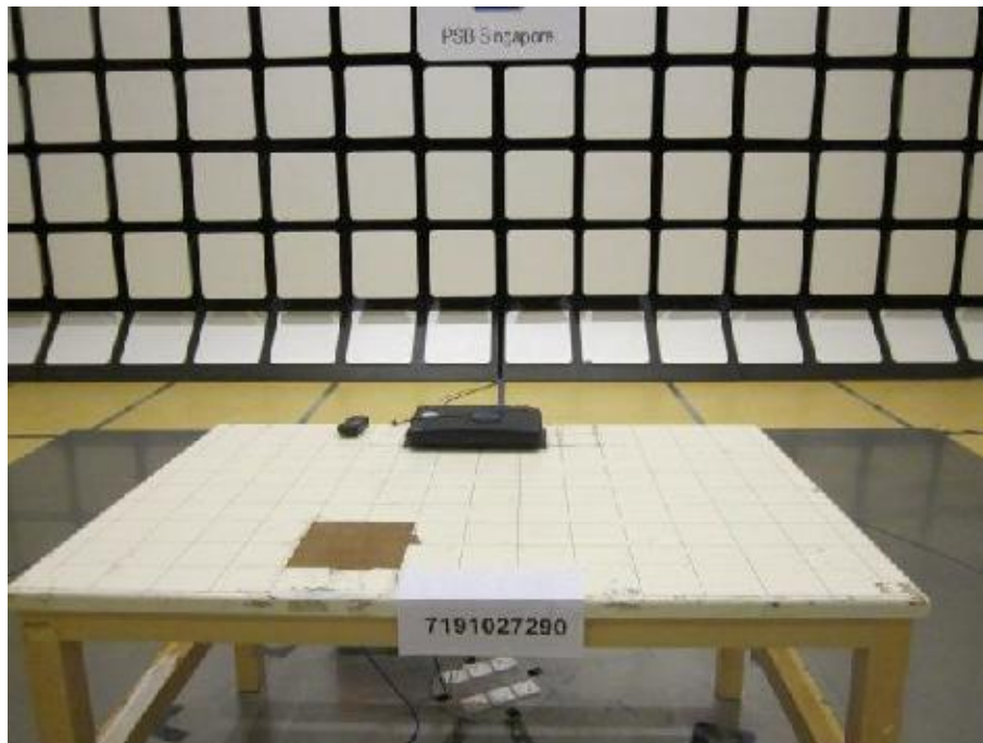
Radiated Spurious Emissions Test Setup (Front View)
