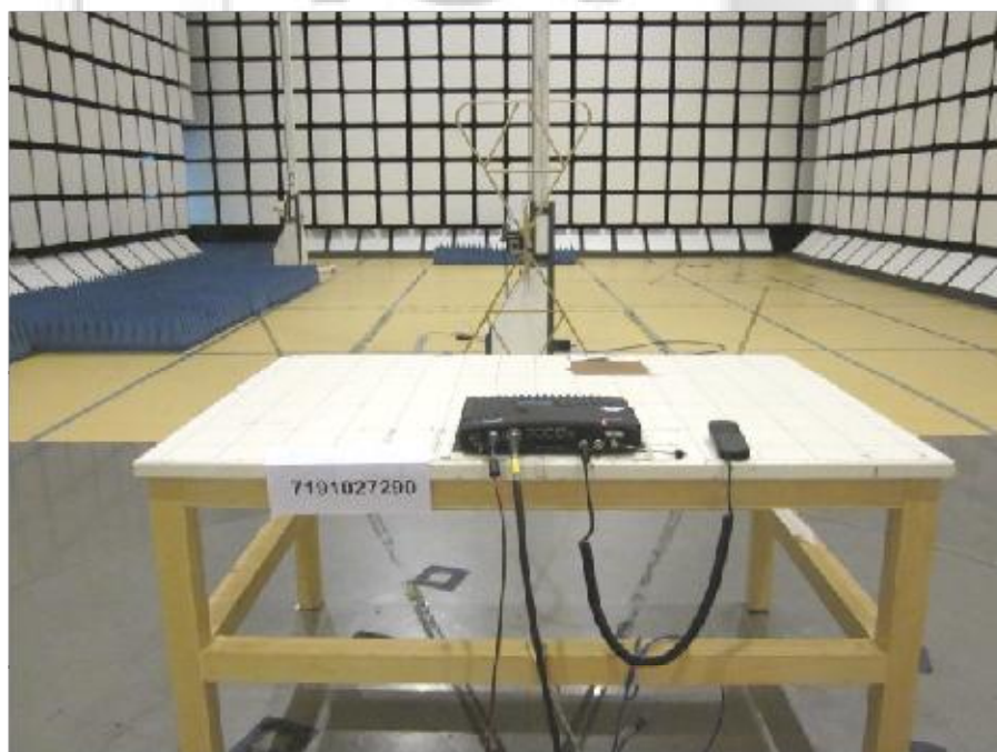
Radiated Emissions Test Setup (Rear View)
