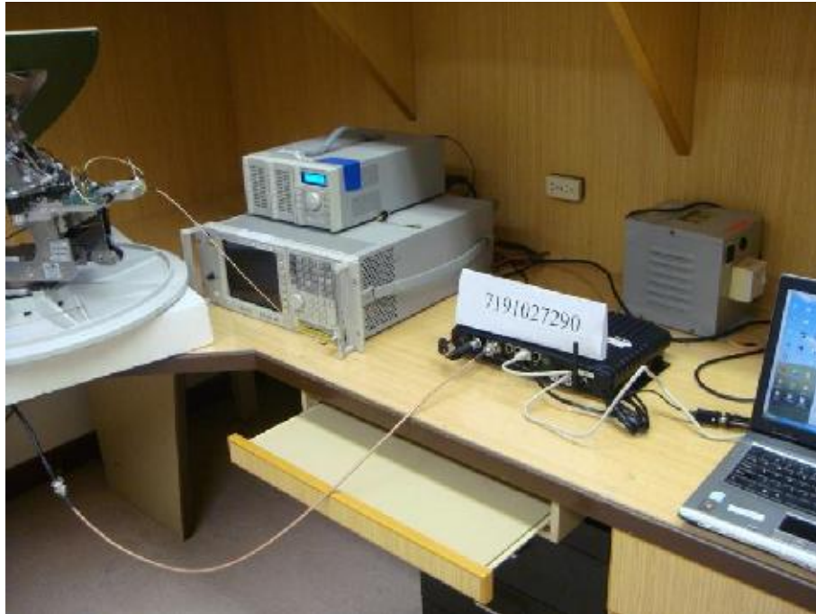
Unwanted Emissions at Antenna Terminal Test Setup
