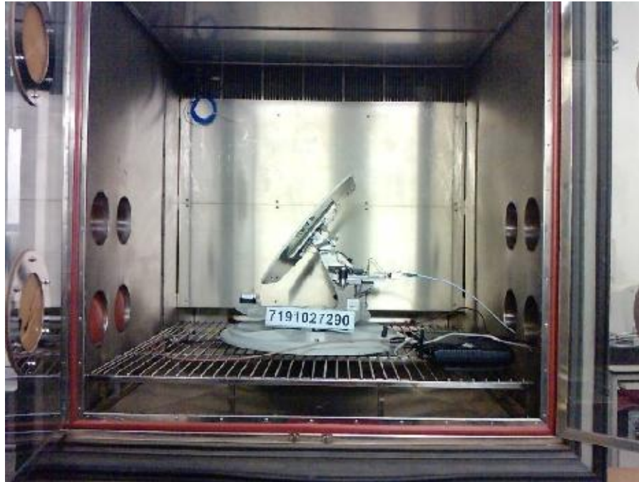
Frequency Stability (Temperature Variation) Test Setup
