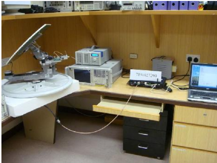
RF Output Power Test Setup
