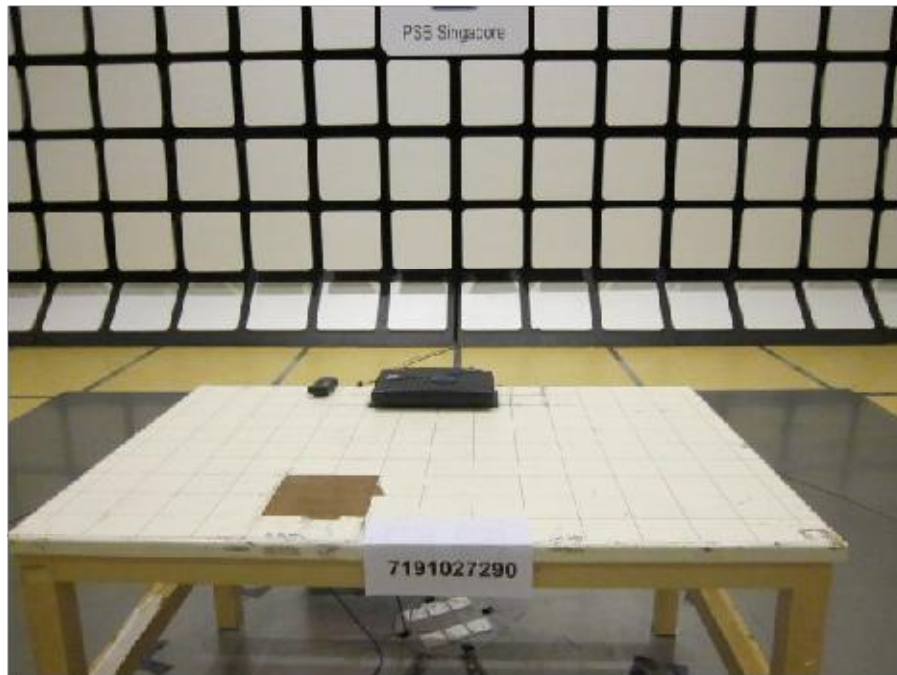
Radiated Emissions Test Setup (Front View)
