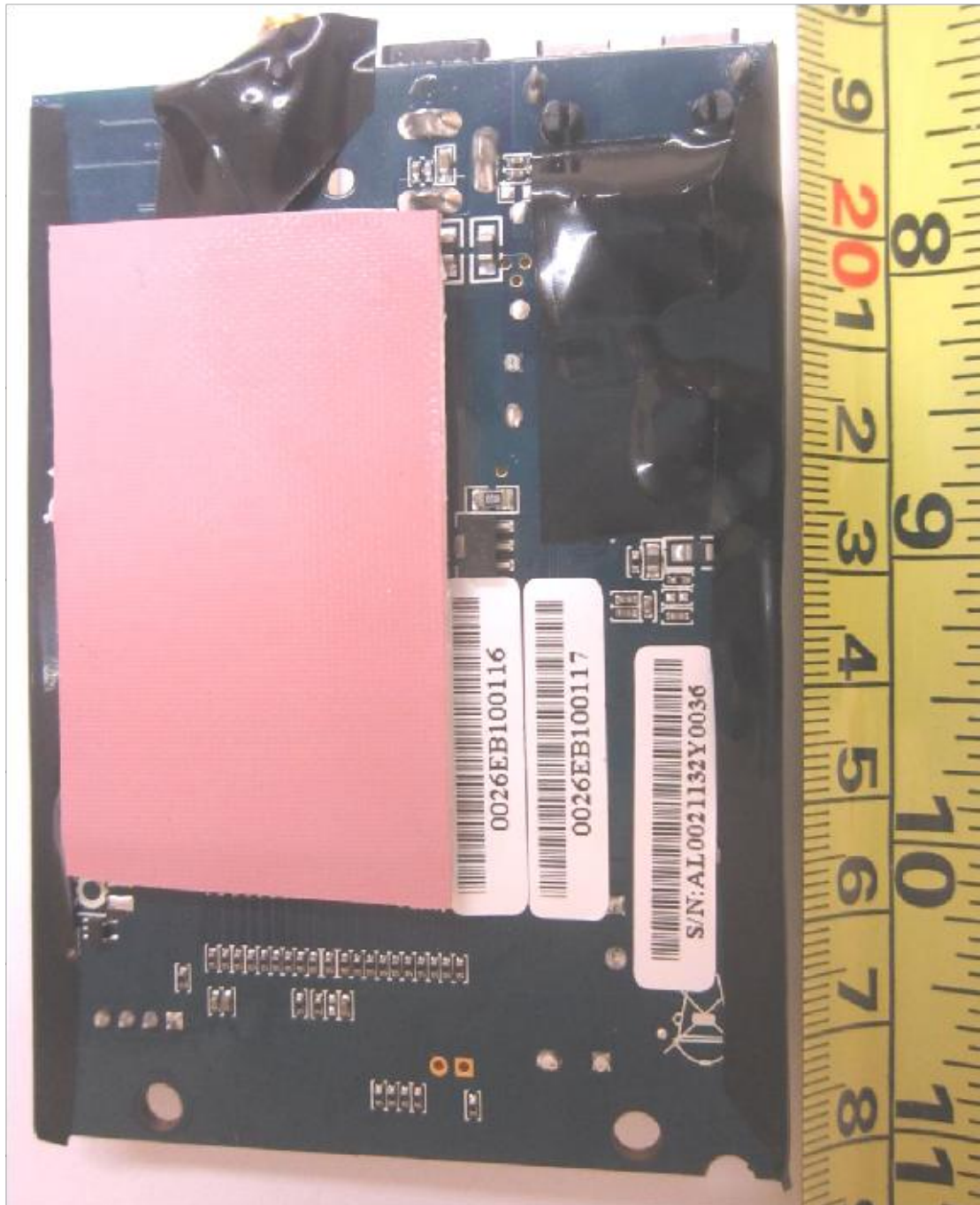
WiFi Module PCB Trace Side
