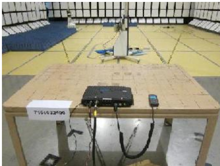
Band Edge Compliance (Radiated) Test Setup
