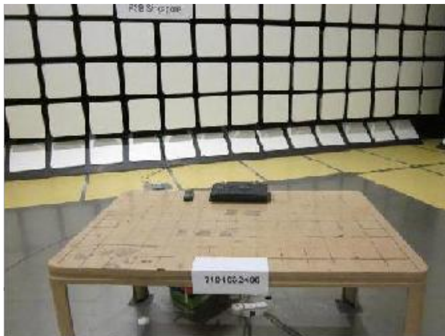
Radiated Emissions Test Setup (Front View)
