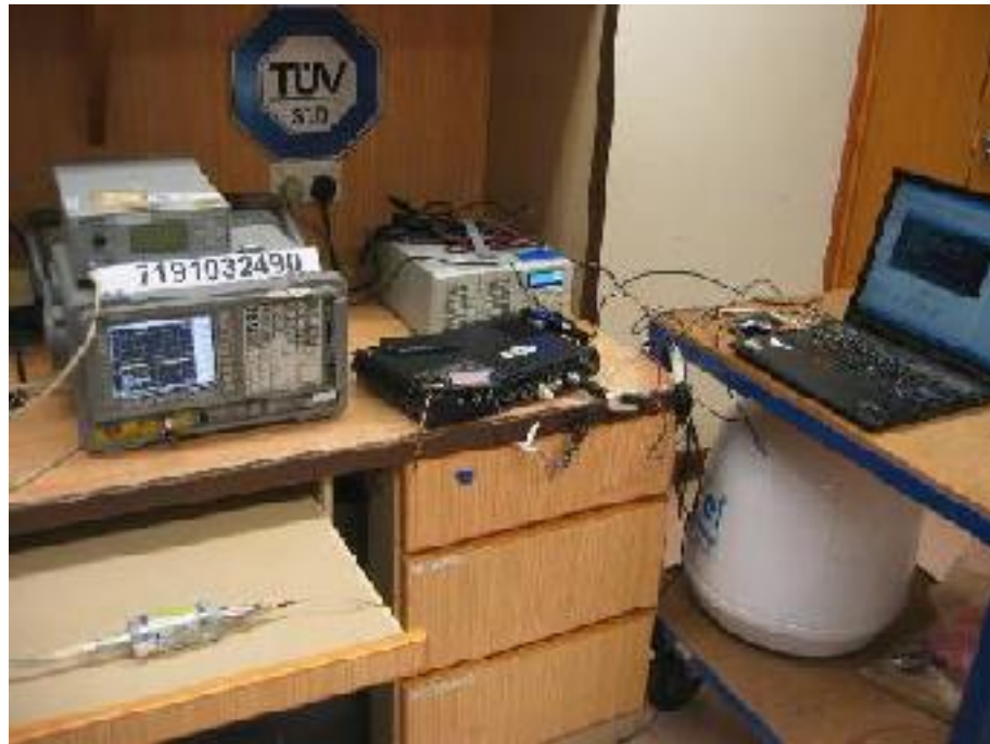
Maximum Peak Power Test Setup
