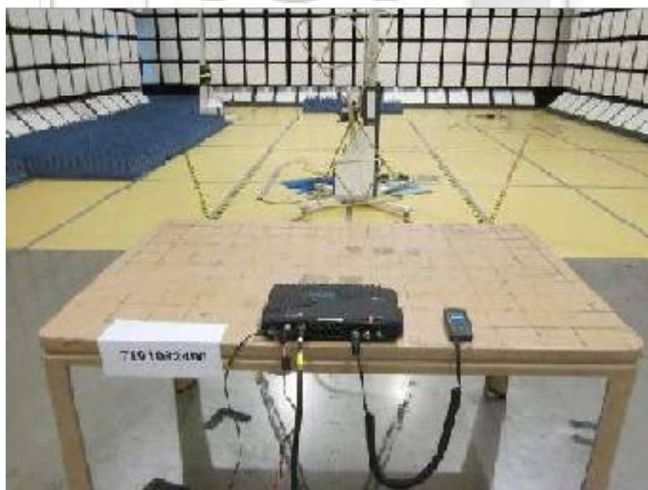
Radiated Emissions Test Setup (Rear View)
