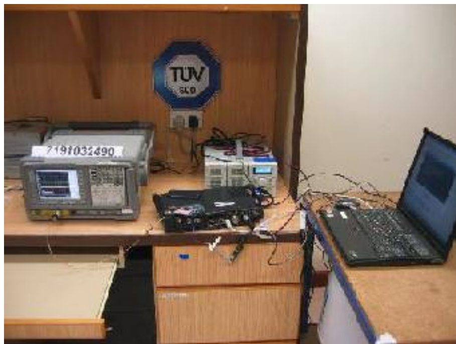
Peak Power Spectral Density Test Setup
