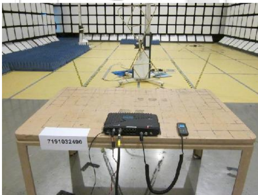
Radiated Emissions Test Setup (Rear View)
