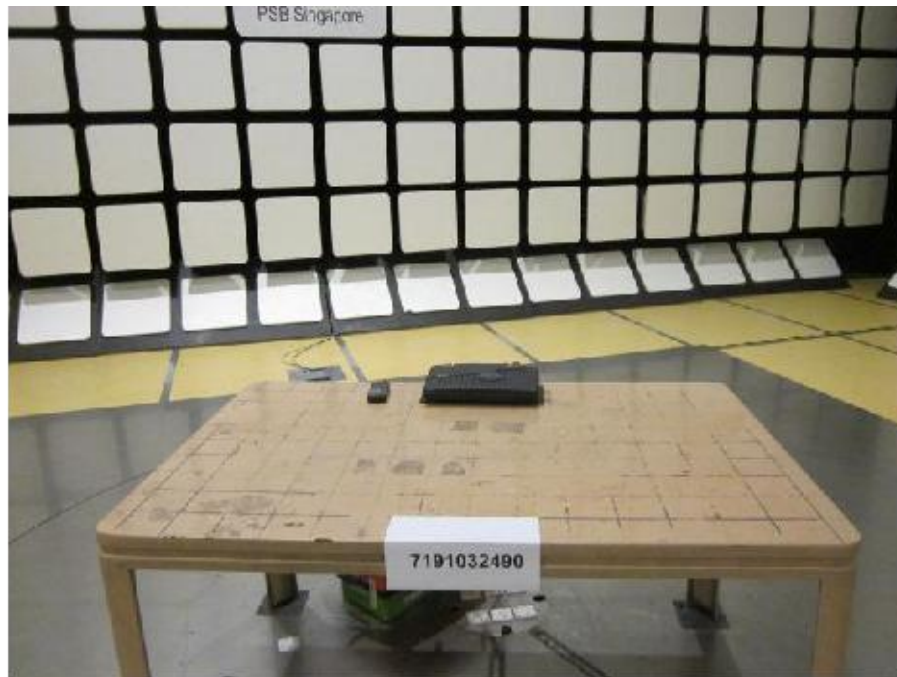
Radiated Spurious Emissions Test Setup (Front View)
