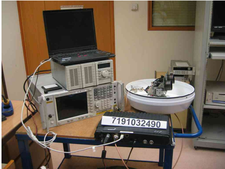
Unwanted Emissions at Antenna Terminal Test Setup
