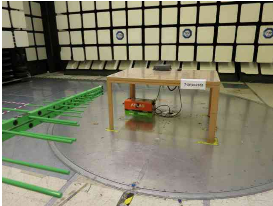
Radiated Spurious Emissions Test Setup (Front View)
