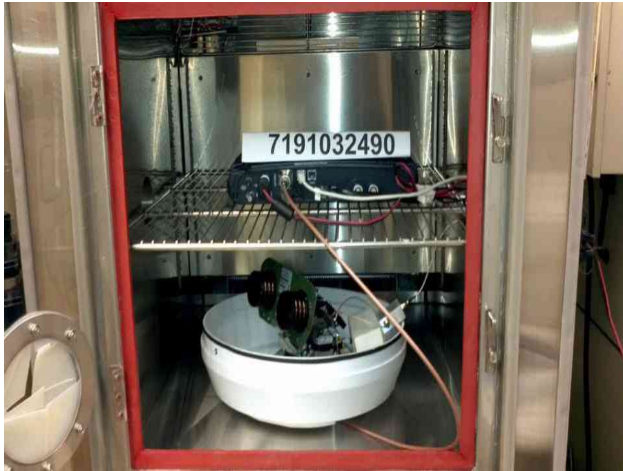
Frequency Stability (Temperature Variation) Test Setup
