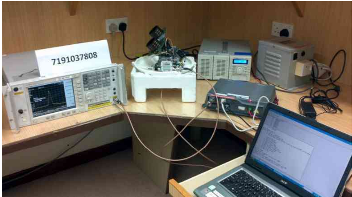
RF Output Power Test Setup
