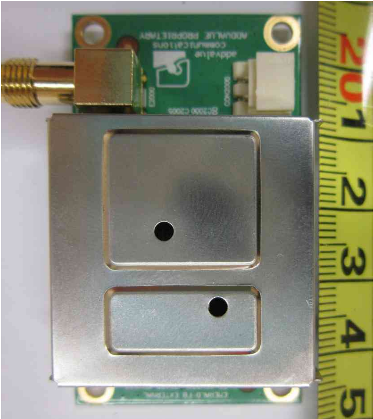
Crystal Board PCB Component Side
