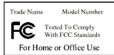
Specifications: Text is black or white in color and is left justified. Labels are silk-screened and shall be "permanently affixed" at a conspicuous location on the EUT.
