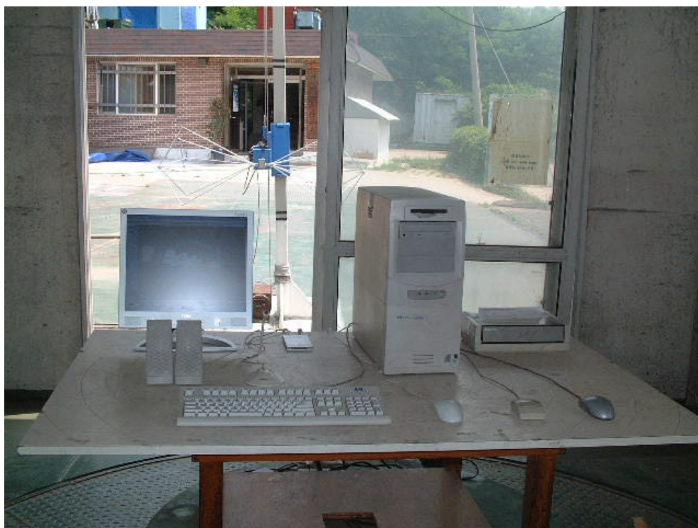
RADIATED EMISSION SETUP PHOTOGRAPH - FRONT VIEW ( 30 - 300 MHz )
