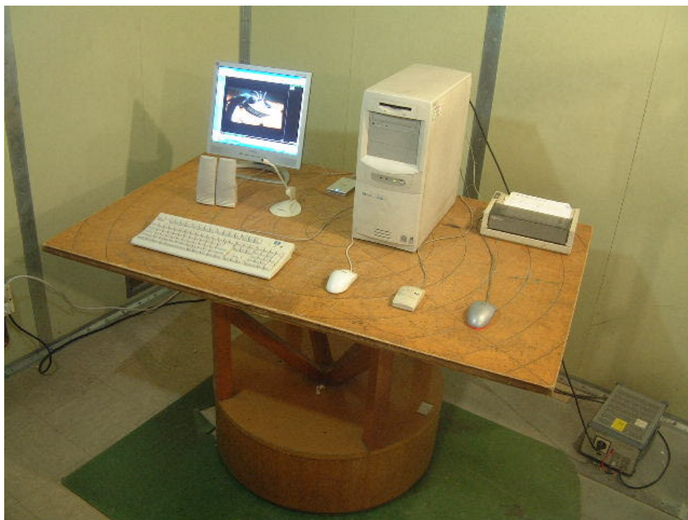
LINE CONDUCTED SETUP PHOTOGRAPH - FRONT VIEW
