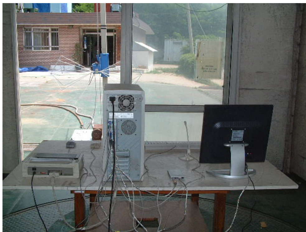
RADIATED EMISSION SETUP PHOTOGRAPH - REAR VIEW ( 30 - 300 MHz )
