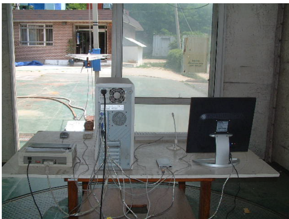
RADIATED EMISSION SETUP PHOTOGRAPH - REAR VIEW ( 300 - 1000 MHz )
