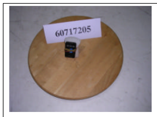
Radiated Open Site Test Set-up
