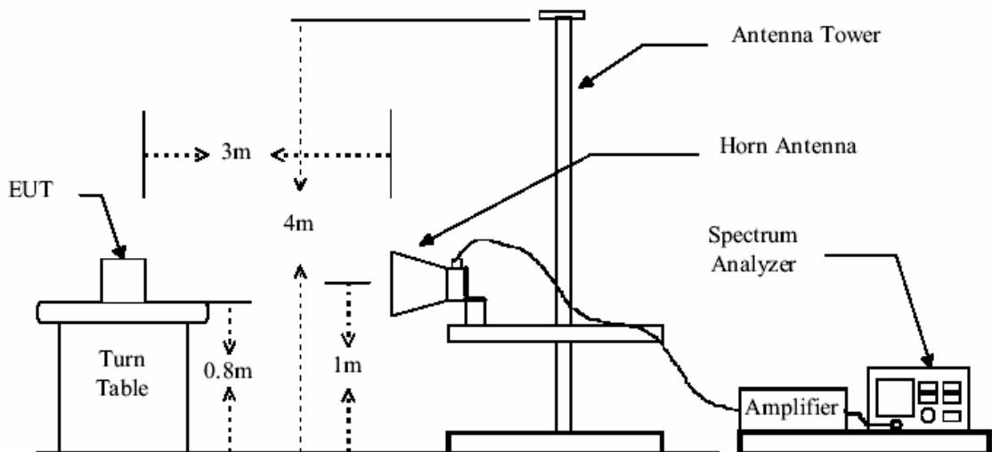
**Test Procedure:** The procedure used was ANSI Standard C63.4-2001. The receiver was scanned from 30MHz to 4.0GHz. When an emission was found, the table was rotated to produce the maximum signal strength. An initial pre-scan was performed for in peak detection mode using the receiver. The EUT was measured for both the Horizontal and Vertical polarities and performed a pre-test three orthogonal planes.
