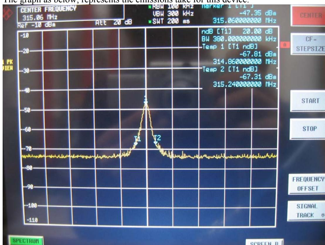
Bandwidth is determined at the points 20 dB down from the modulated carrier is 380 KHz , it's less than the limit: 0.25% of the center frequency = 787.5 KHz.
