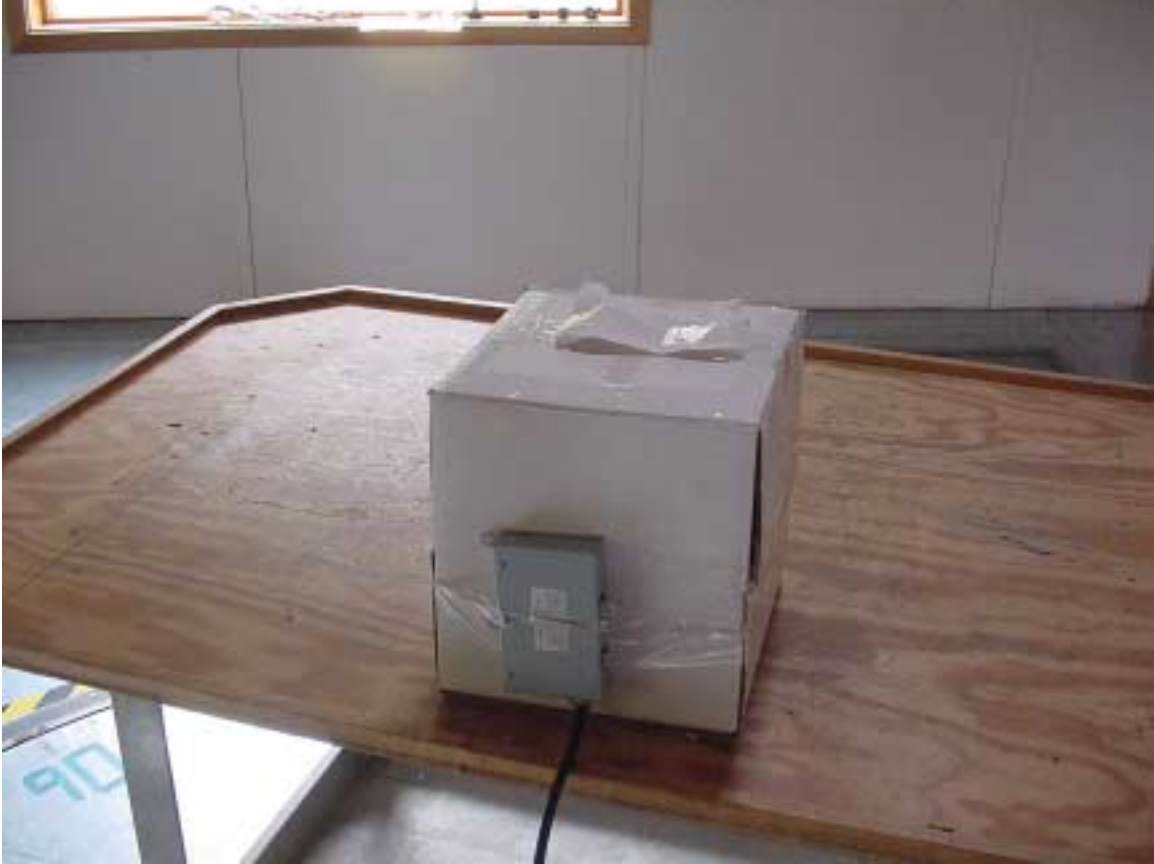
QNG-02001 Photo showing Radiated OATS setup in worst case orthogonal plane. The cardboard box is empty and dry. The table is a Rubbermaid plastic cart.
