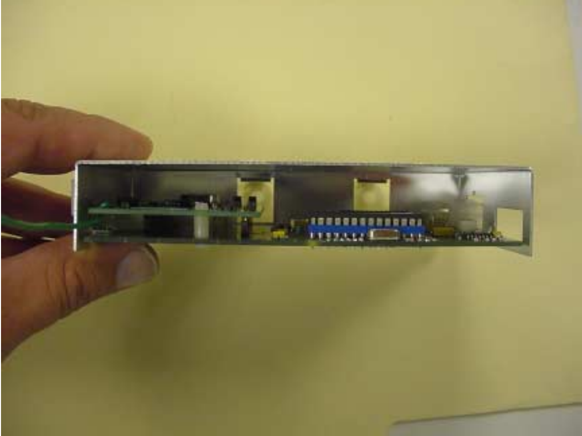
QNG-02001 Photo of side view showing layout of boards inside EUT.
