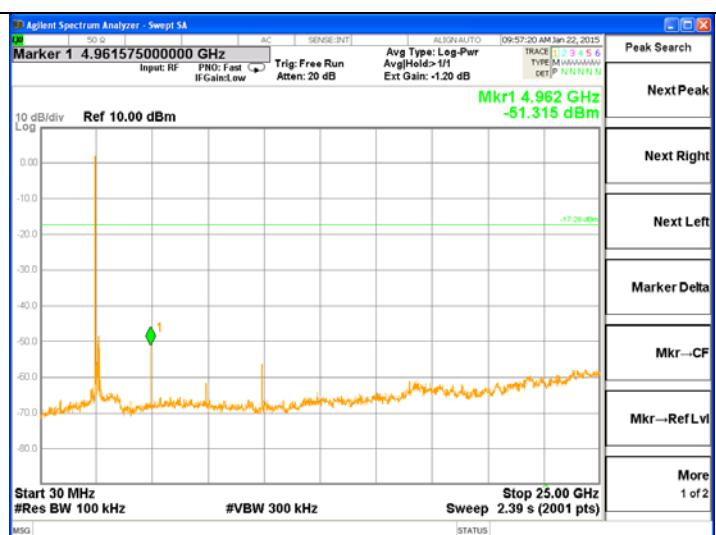
Conducted Spurious Emission - EDR( $\pi/4$ -DQPSK)
