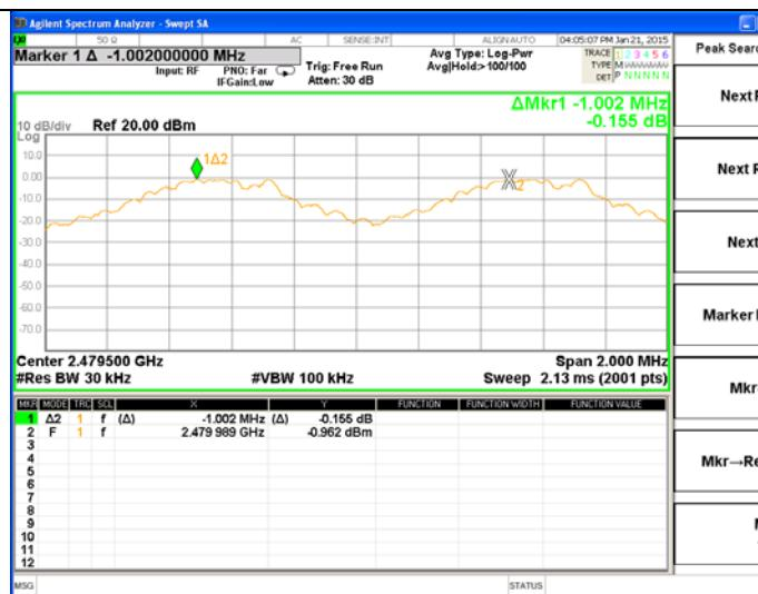
Hopping Channel Separation - EDR( $\pi/4$ -DQPSK)
