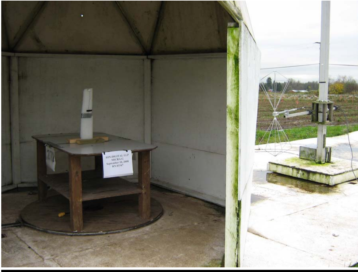
Figure 2: Emissions Test Set up
