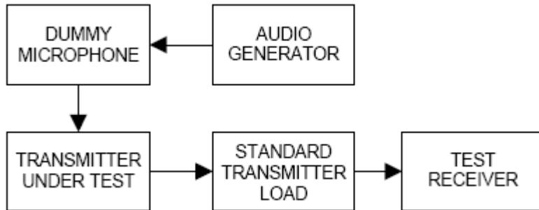
Test at five different modulating frequencies (100Hz, 300Hz, 500Hz, 1KHz, 2.5kHz, 5kHz), the output level of the audio generator was varied up to 1V and the FM deviation level was recorded.
