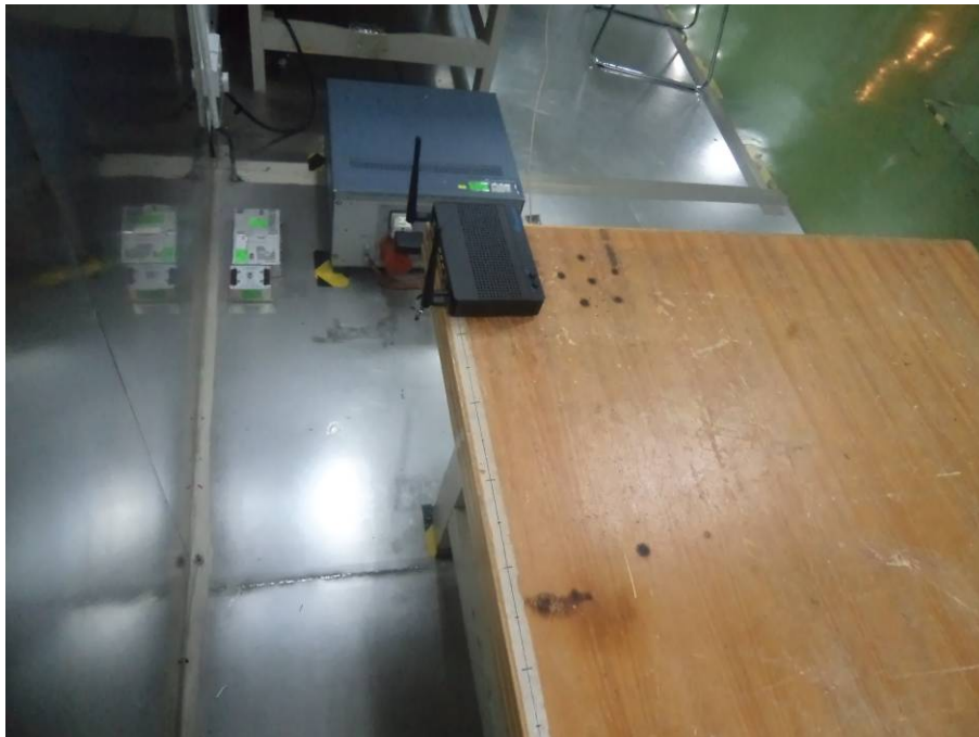
Conduction Emissions - Side View
