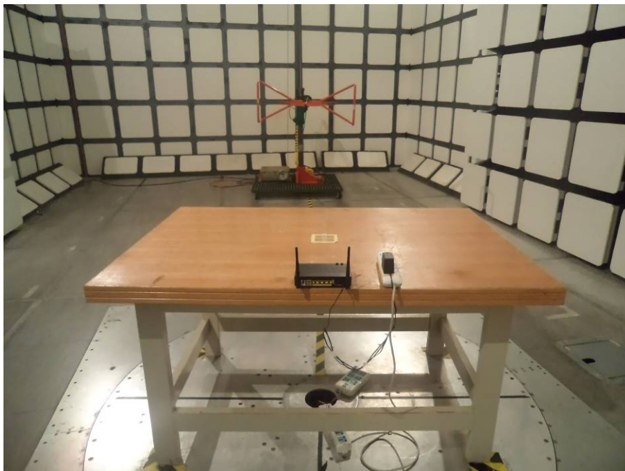
Radiated Emissions – Rear View (Below 1 GHz)
