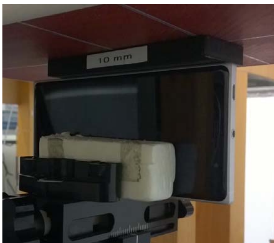
Photo of the device positioned for WR mode measurement – left edge facing phantom. The spacer was removed before the start of the measurements.
