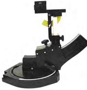
Device holder supplied by SPEAG
