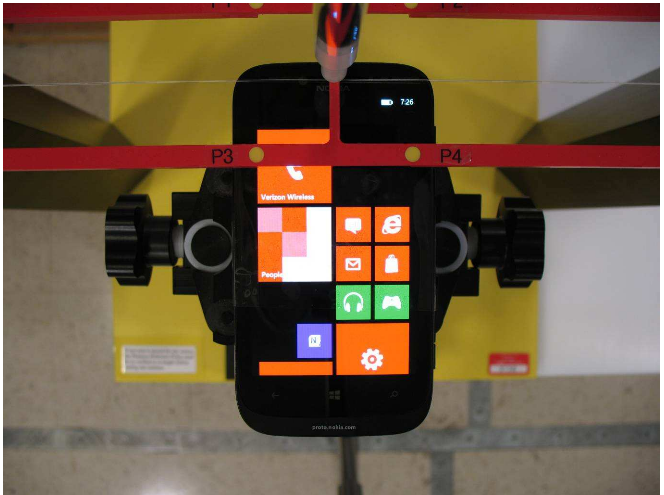
Figure 5: Test Setup Photograph – Near Field Emissions Test Showing EUT Centered on Test Arch
