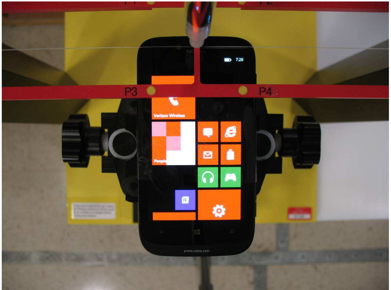
Figure 3: Test Setup Photograph – Near Field Emissions Test Showing EUT Centered on Test Arch
