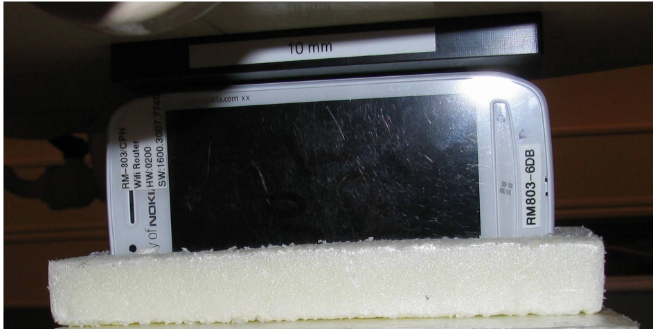
Photo of the device positioned for WR mode measurement – right edge facing phantom. The spacer was removed before the start of the measurements.
