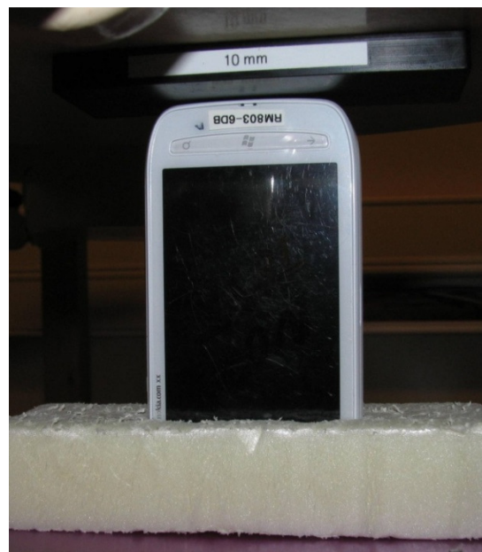
Photo of the device positioned for WR mode measurement – bottom edge facing phantom. The spacer was removed before the start of the measurements.
