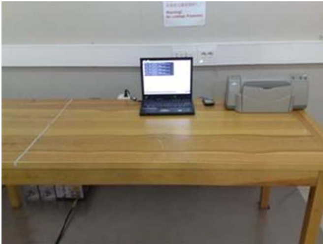
Picture 5. FCC Part 15B AC powerline conducted emissions, computer peripherals, measure from PC charger
