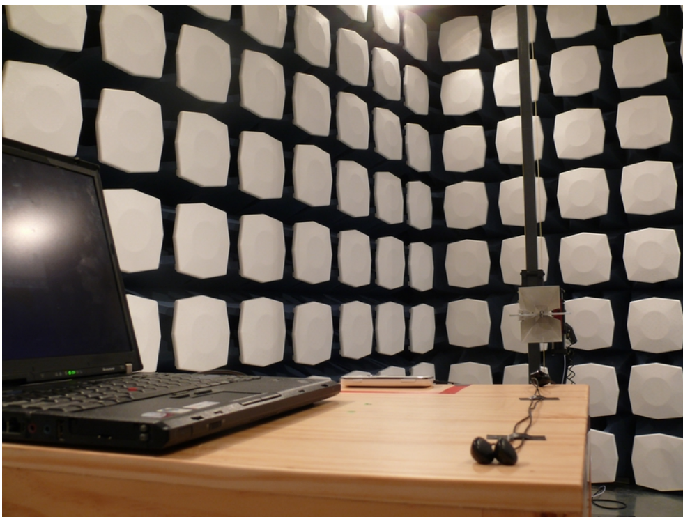
Picture 1: Radiated Emission Test Setup
