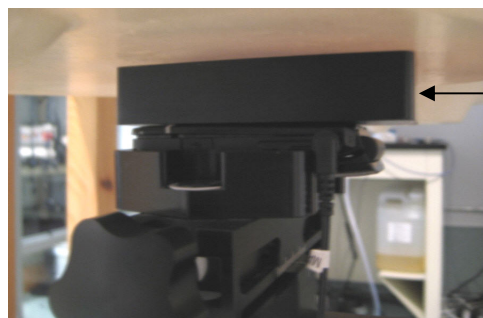
Photo of device positioned for Body SAR measurement. The spacer was removed for the tests.
