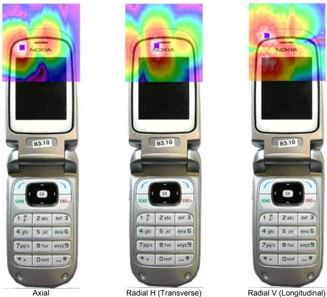
Figure 13-3 T-Coil Scan Overlay Magnetic Field Distributions
