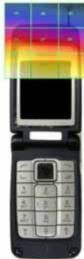
Figure 28 Sample H-field Scan Overlay
