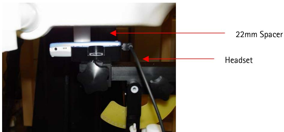
Note: the 22mm spacer was removed before the SAR measurement.
