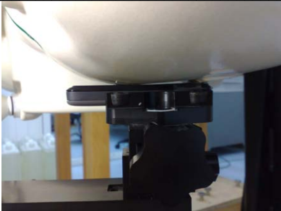
Photo of the device in “cheek” position
