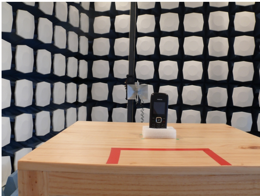
Picture 1: Radiated Spurious Emissions Test setup
