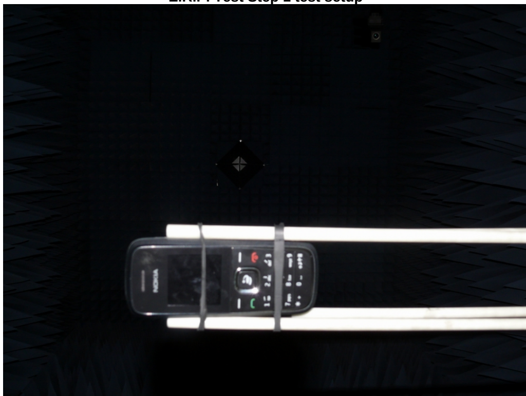
E.R.P. Test Step 2 test setup Picture 2: ERP Test setup
