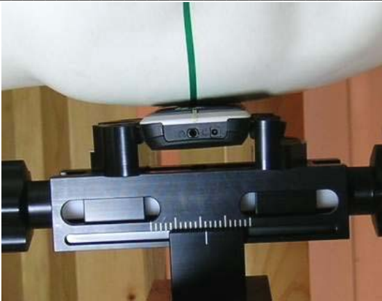
Photo of the device in "cheek" position
