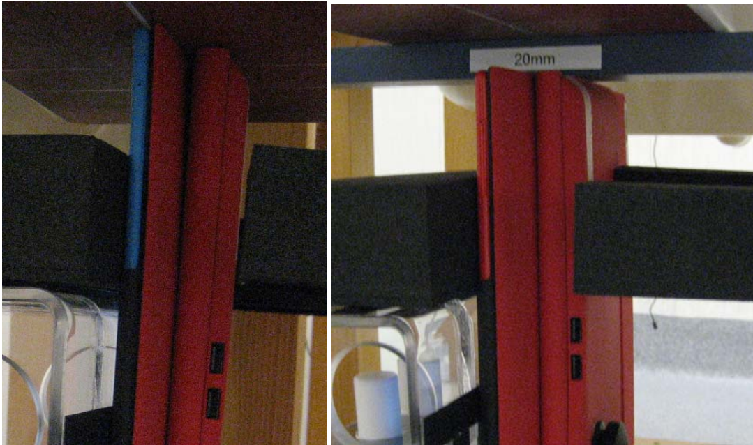
Photo of the device with SU-42 Smart cover (tablet mode) positioned for left edge facing phantom. The spacer was removed before the start of the measurements.
