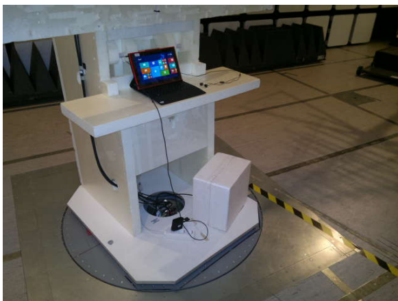
Picture 2. FCC Part 15B Radiated emissions, Smart cover
