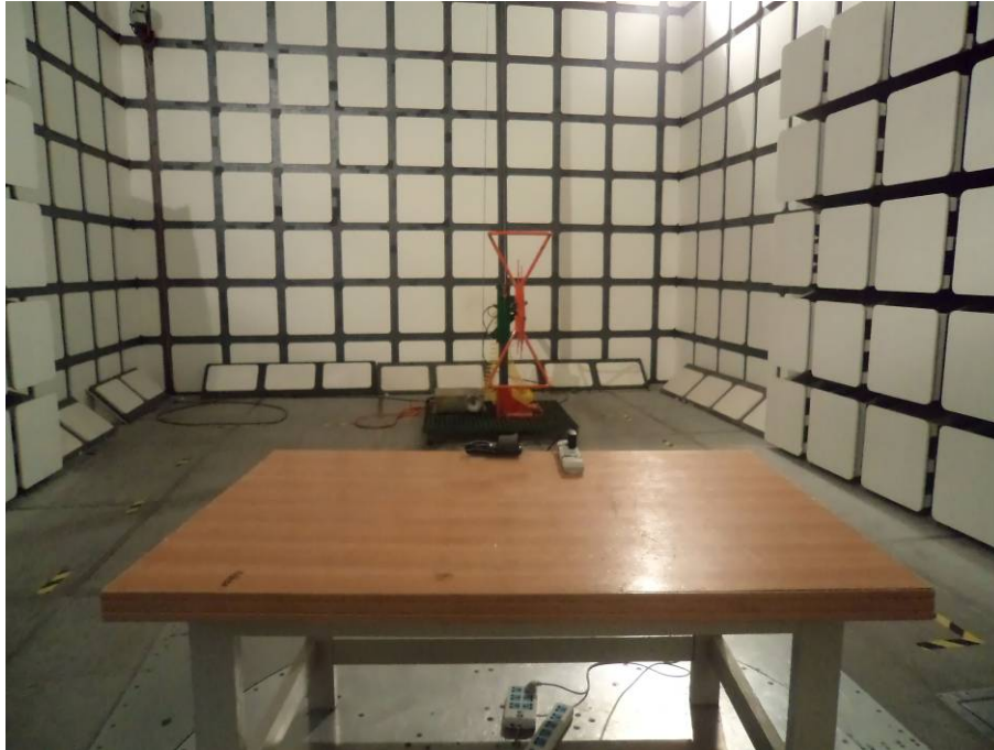
Below 1 GHz: Radiated Emissions – Front View
