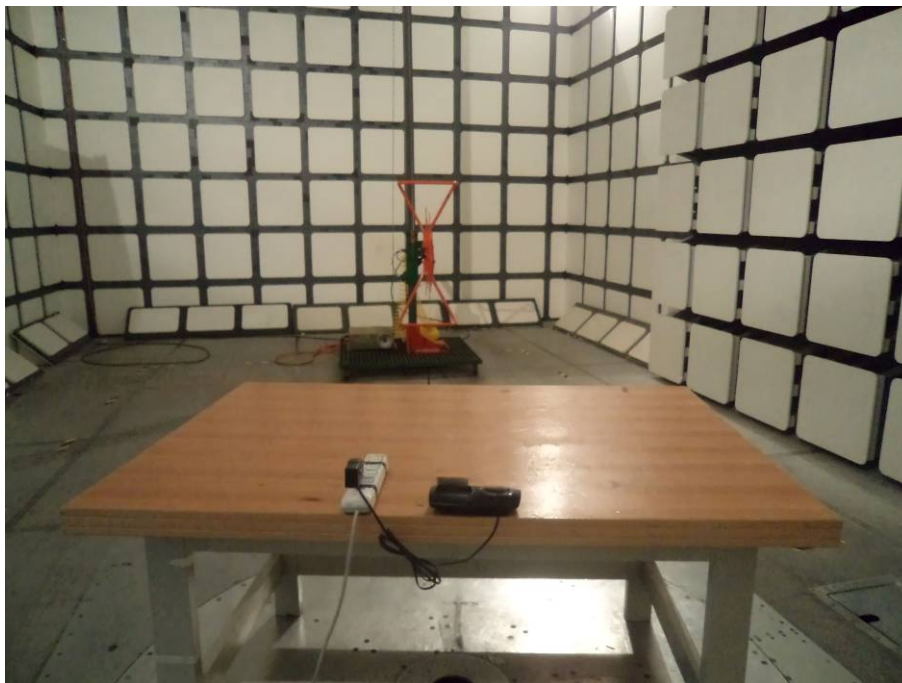
Below 1 GHz: Radiated Emissions – Rear View
