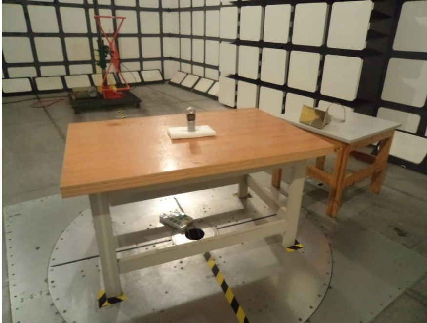
Radiated Emissions View (Below 1 GHz)
