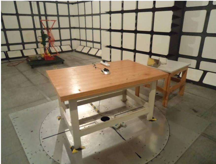
Radiated Emissions View (Below 1 GHz)
