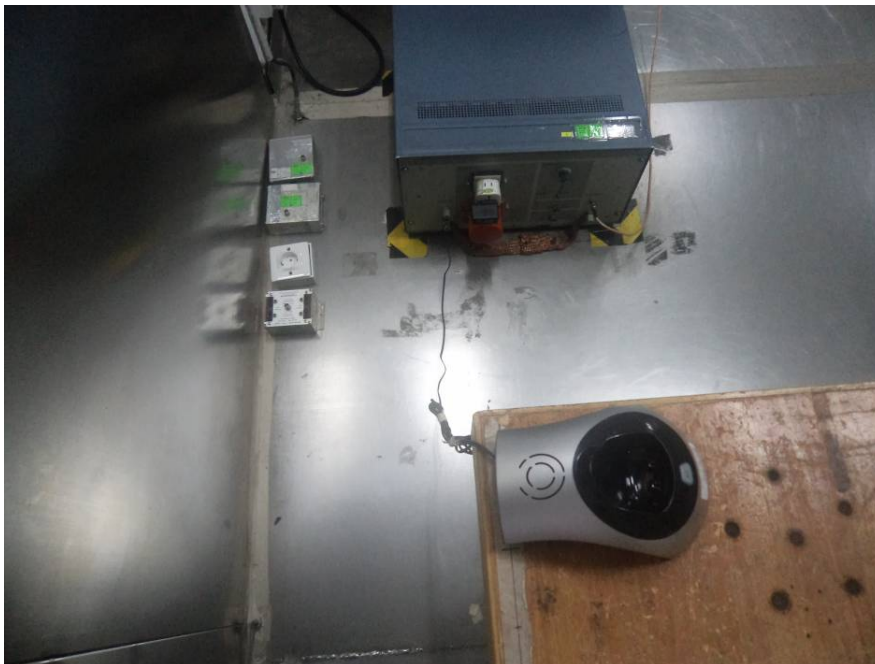
Conducted Emissions - Side View
