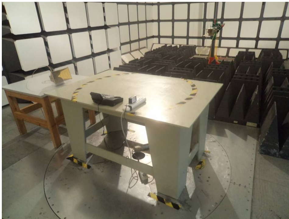
Radiated Emissions - Rear View (Above 1 GHz)
