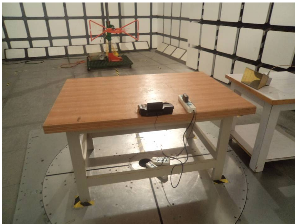
Radiated Emissions - Rear View (Below 1 GHz)
