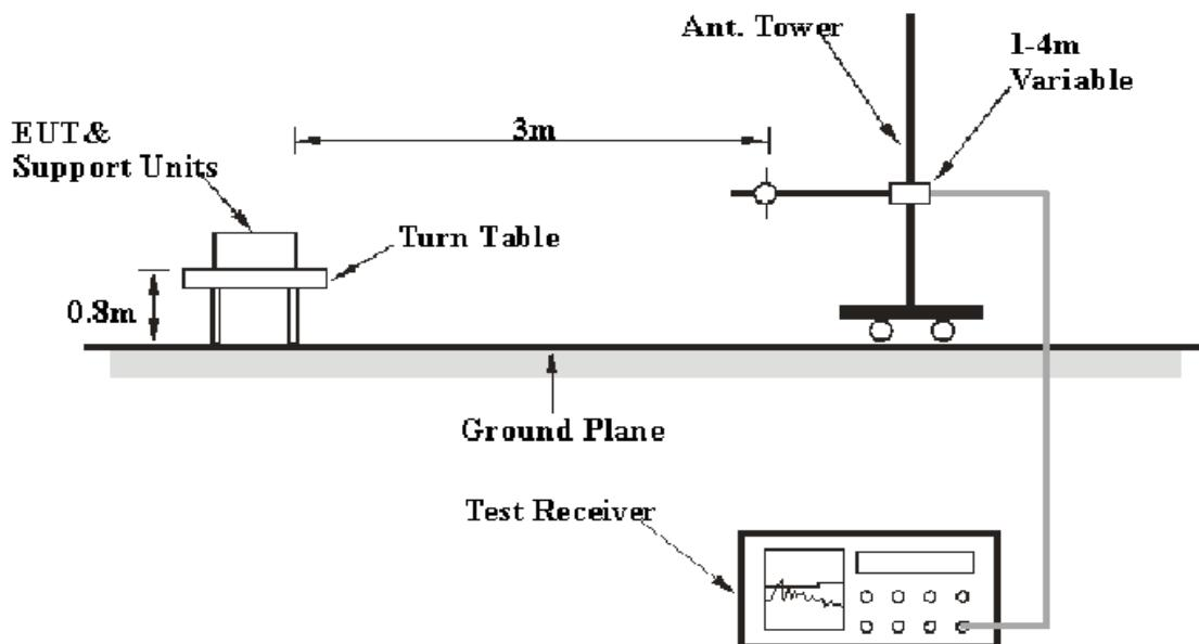
The radiated emission tests were performed in the 3 meters chamber test site, using the setup accordance with the ANSI C63.17 - 2006. The specification used was the FCC 15§ 15.319(g).
