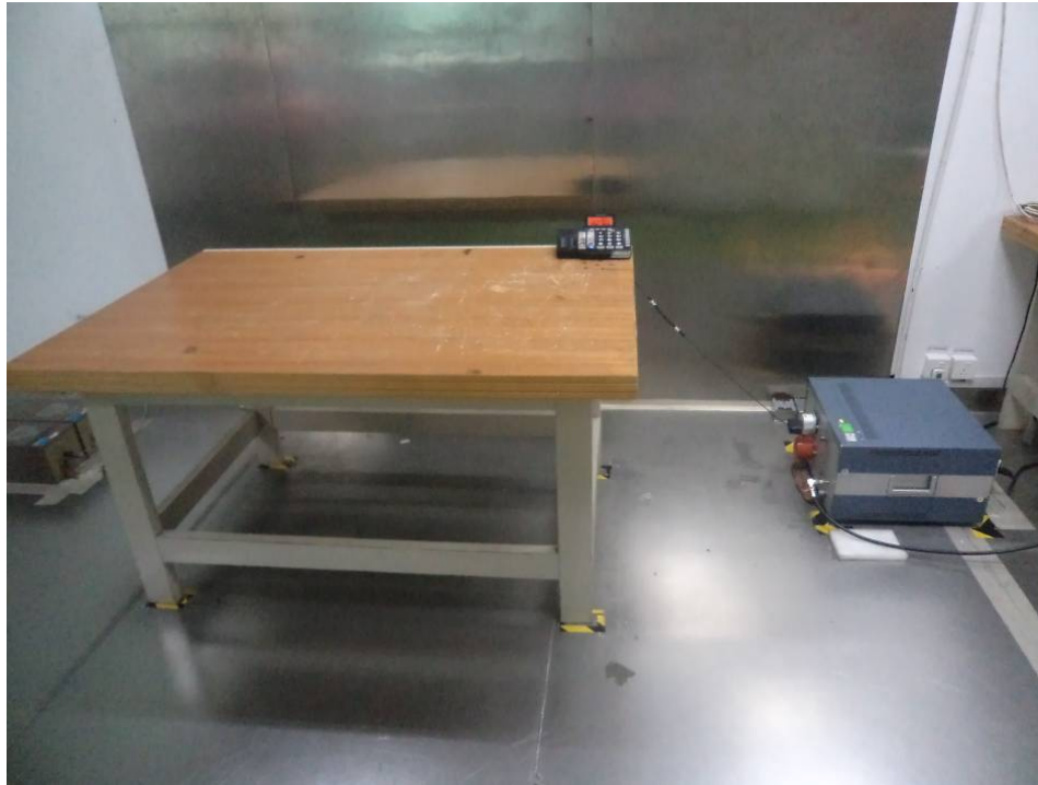
Conducted Emissions - Side View
