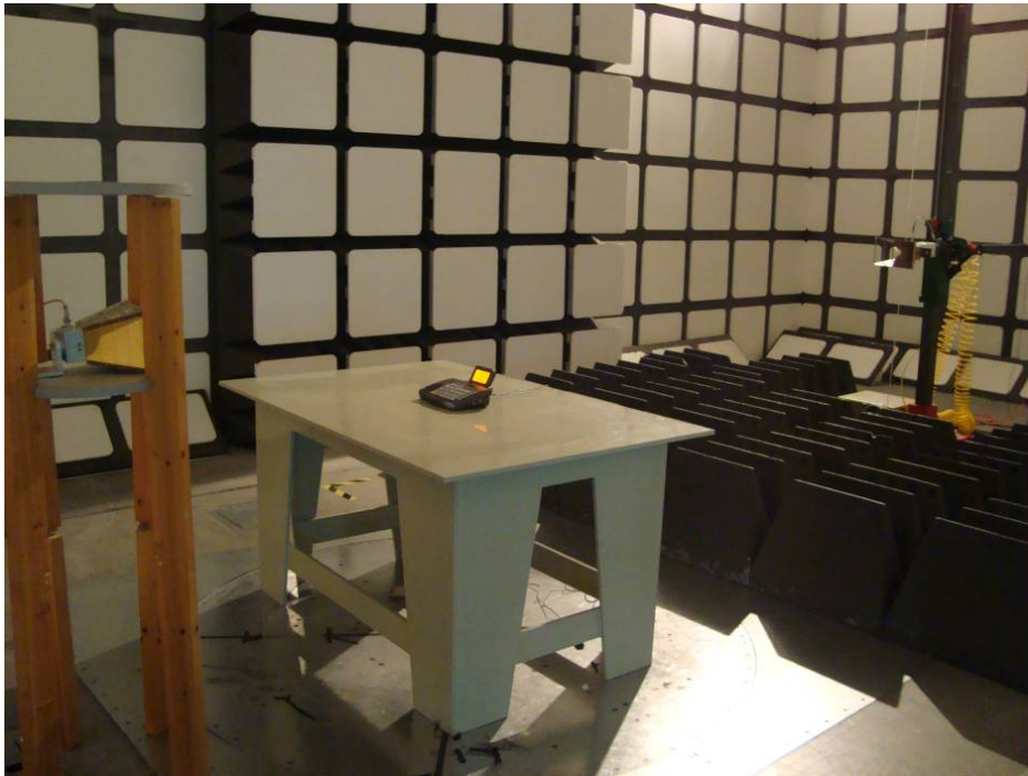
Spurious Emissions - Rear View (Above 1 GHz, transmitting mode)
