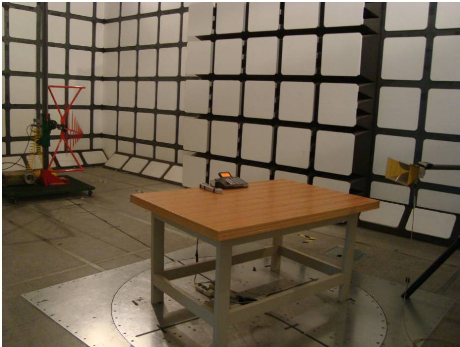
Radiated Emissions - Rear View (30-1000 MHz, transmitting mode)
