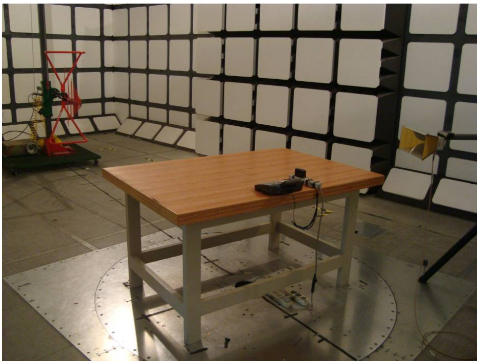
Radiated Emissions - Rear View (30-1000 MHz, transmitting mode)
