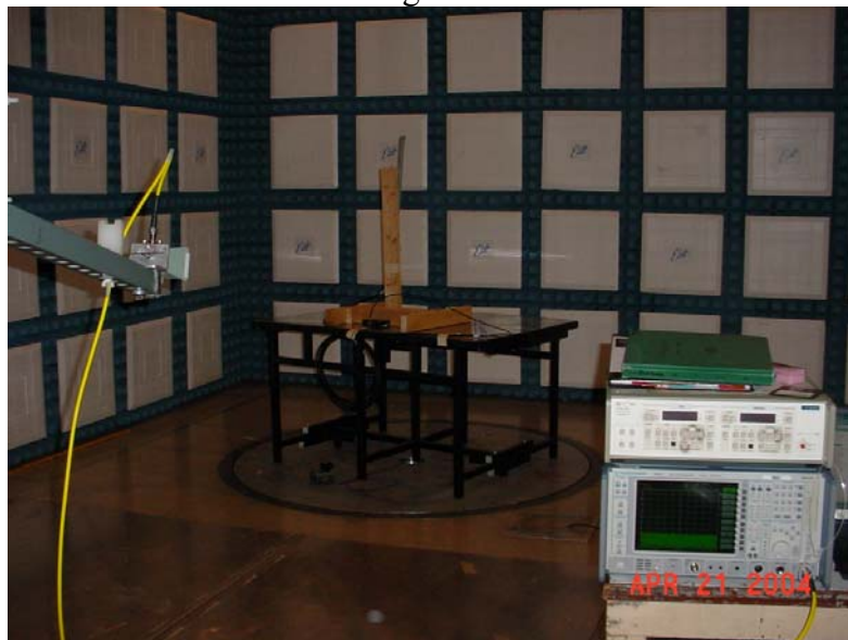
Test Setup for Measurement of Radiated Emissions from a Pacific Wireless Model OD-24-9 Omni Antenna and 29 feet of Times Microwave LMR-400 Cable
