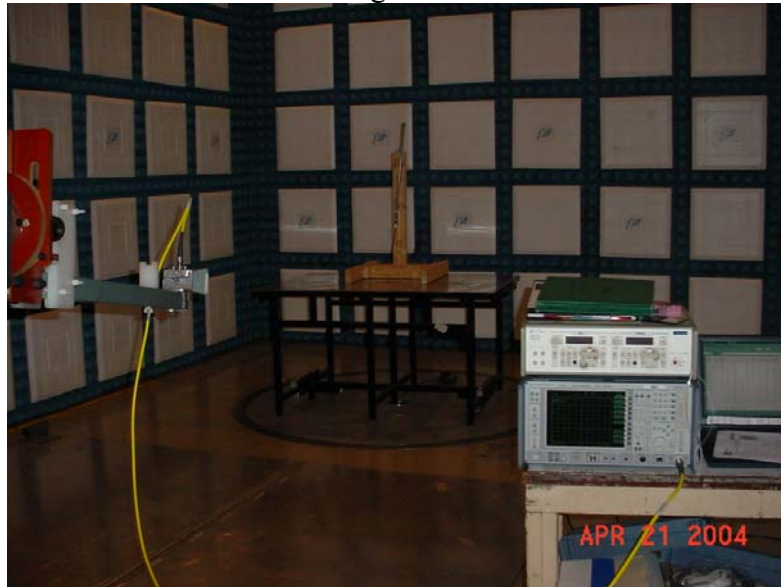
Test Setup for Measurement of Radiated Emissions from a Pacific Wireless Model OD-24-9 Omni Antenna and 4 feet of Times Microwave LMR-195 Cable
