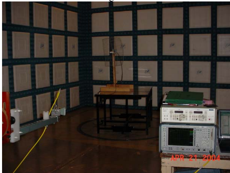
Test Setup for Measurement of Radiated Emissions from a Pacific Wireless Model PMANT-19-HD-PF1 Parabolic Grid Antenna and 29 feet of Times Microwave LMR-400 cable
