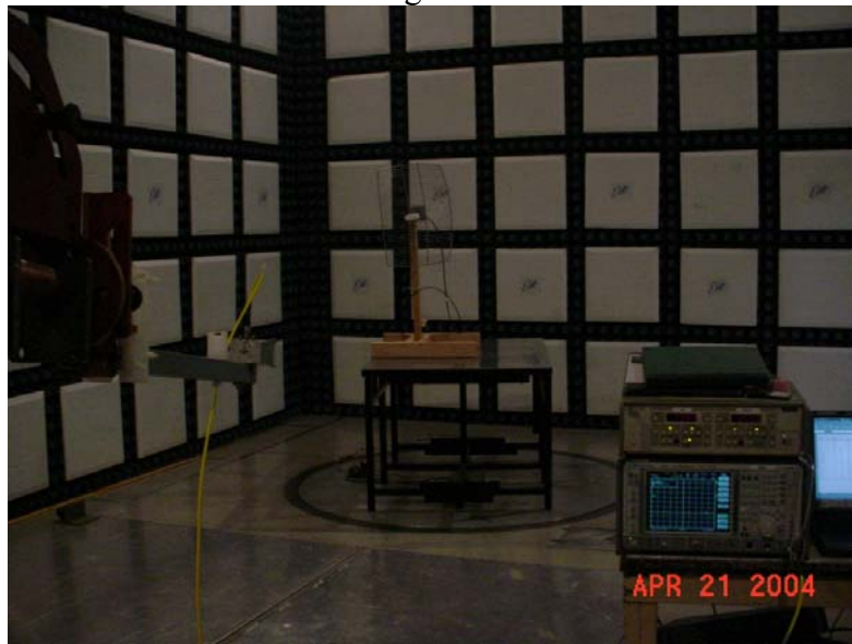
Test Setup for Measurement of Radiated Emissions from a Pacific Wireless Model PMANT-19-HD-PF1 Parabolic Grid Antenna and 4 feet of Times Microwave LMR-195 Cable
