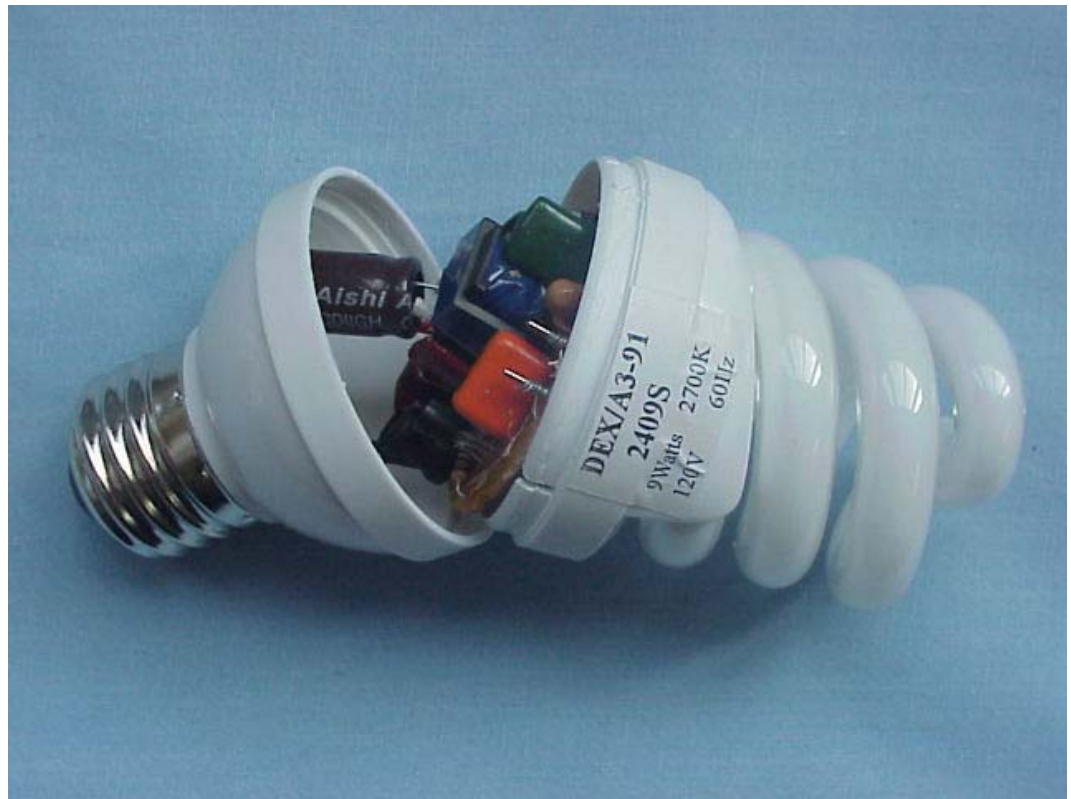
FIGURE 1 SELF-BALLASTED FLUORESCENT LAMP (M/N: DEX/A3-91) COVER REMOVED
