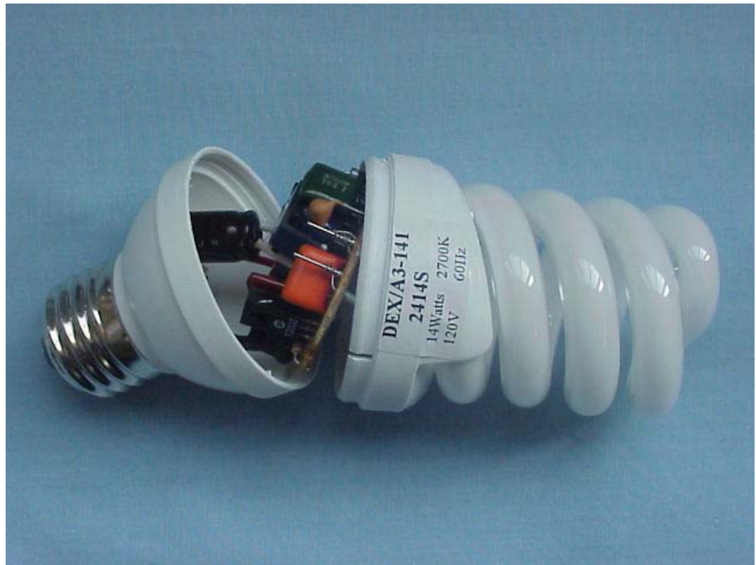
FIGURE 7 SELF-BALLASTED FLUORESCENT LAMP (M/N: DEX/A3-141) COVER REMOVED
