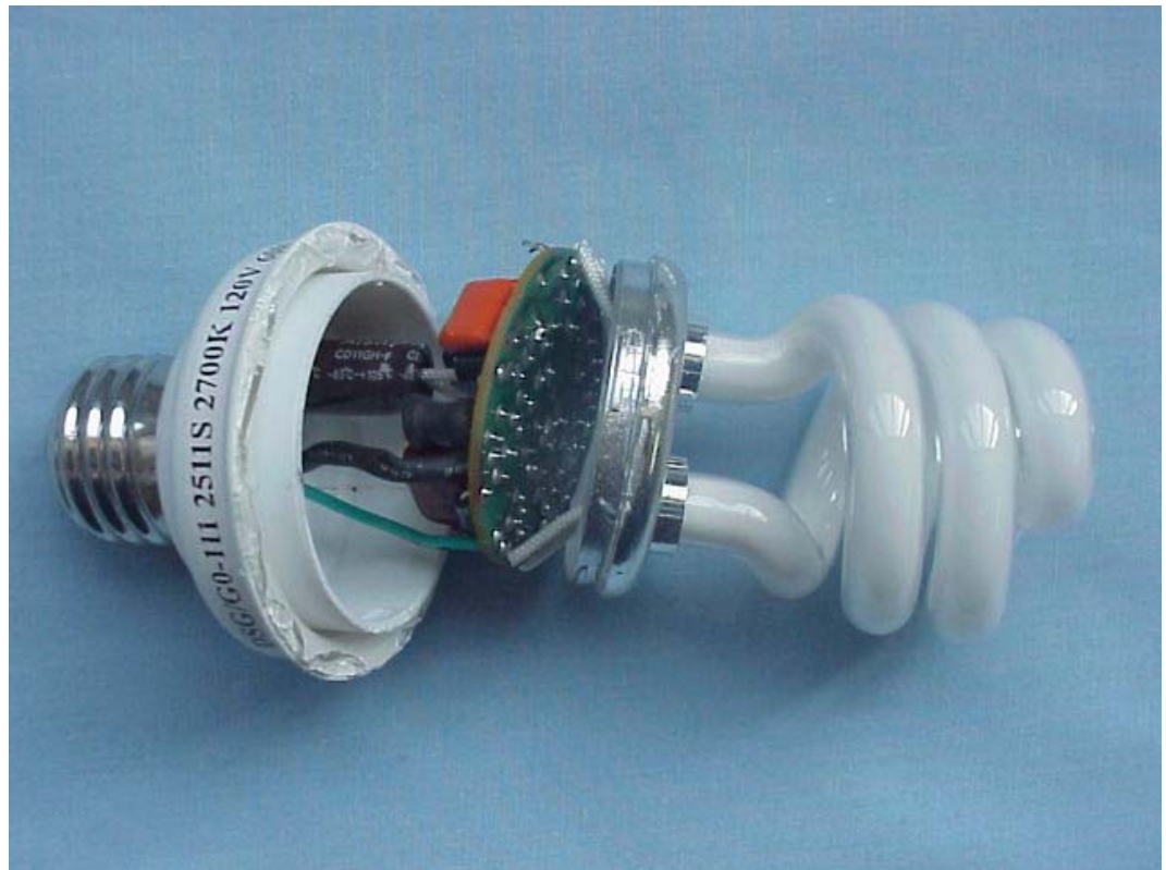
FIGURE 19 SELF-BALLASTED FLUORESCENT LAMP (M/N: DSG/G0-111) COVER REMOVED
