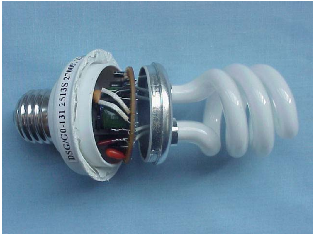
FIGURE 22 SELF-BALLASTED FLUORESCENT LAMP (M/N: DSG/G0-131) COVER REMOVED
