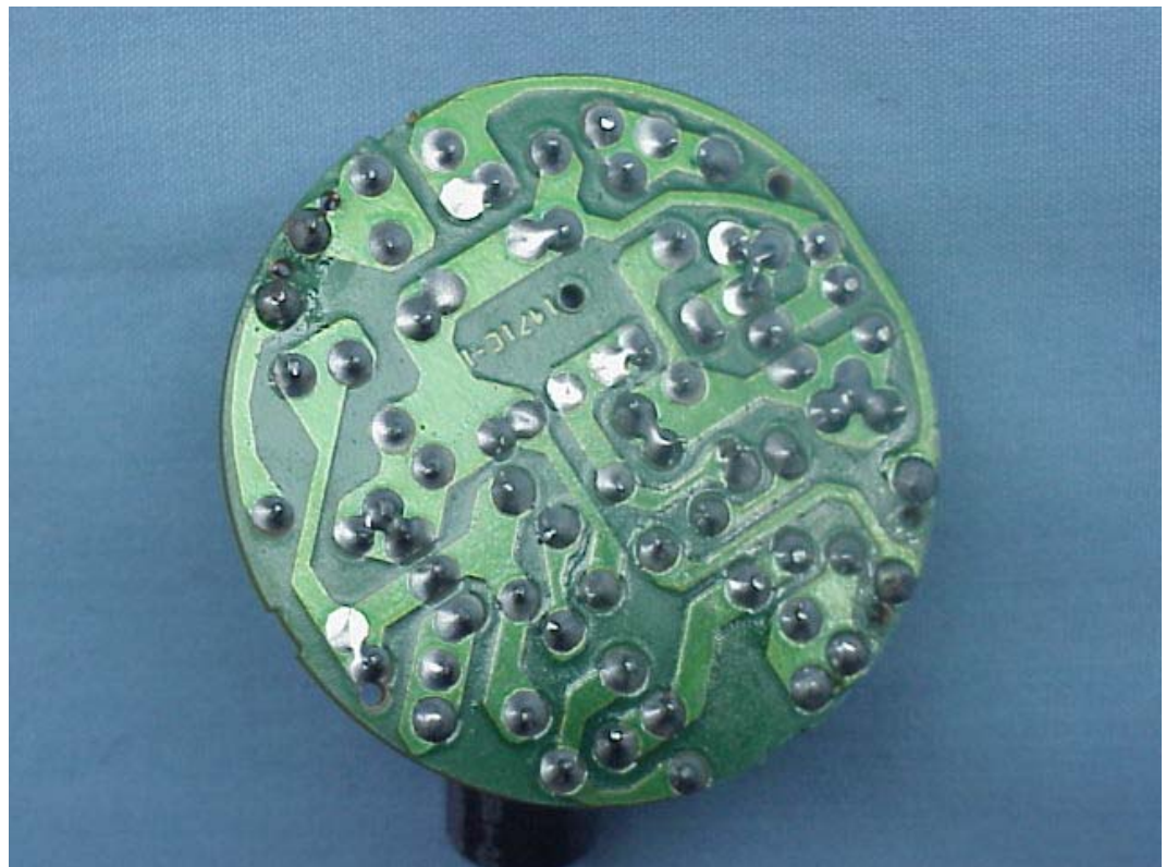
FIGURE 21 SELF-BALLASTED FLUORESCENT LAMP (M/N: DSG/G0-111) PCB BOARD (SOLDERED SIDE)
