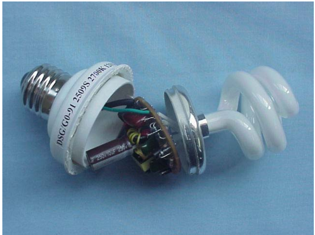
FIGURE 16 SELF-BALLASTED FLUORESCENT LAMP (M/N: DSG/G0-91) COVER REMOVED
