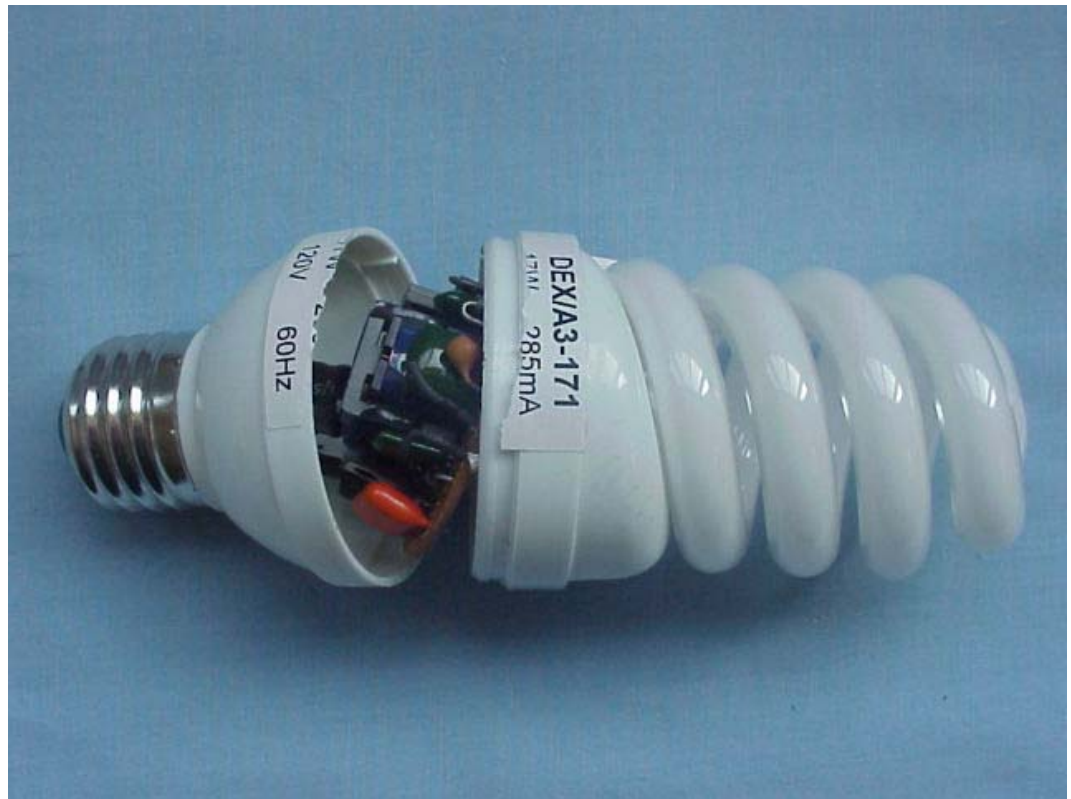
FIGURE 10 SELF-BALLASTED FLUORESCENT LAMP (M/N: DEX/A3-171) COVER REMOVED
