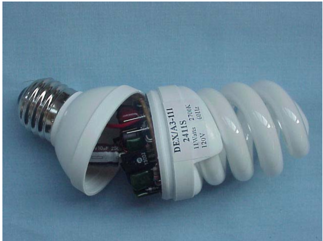
FIGURE 4 SELF-BALLASTED FLUORESCENT LAMP (M/N: DEX/A3-111) COVER REMOVED
