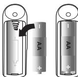
Put the battery into the compartment. Pay attention to the polarity.
