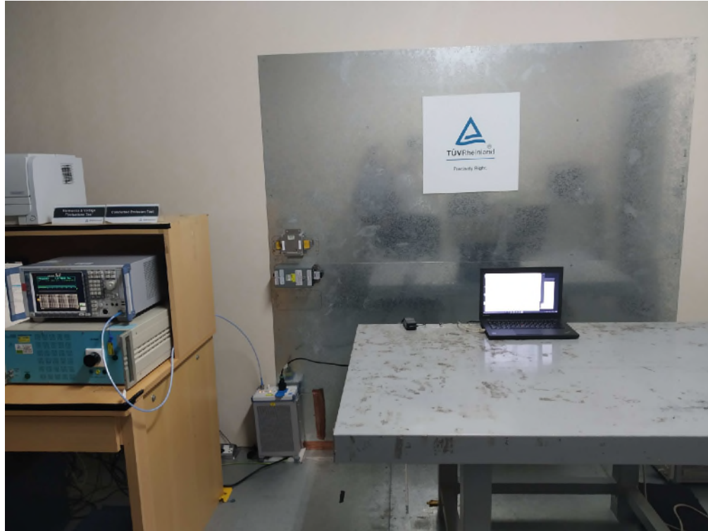
Photograph 7: Set-up for Mains Conducted testing (Front View)
