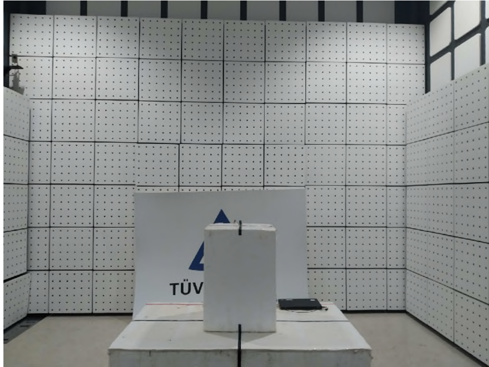
Photograph 2: Set-up for Spurious Emissions (Front View 2)
