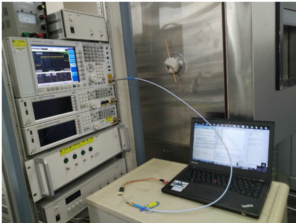
Photograph 5: Set-up for Conducted testing (View 1)
